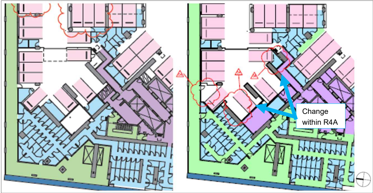
Figure 5 | Comparison of the approved (left) and proposed (right) Level B2 showing removal of two storage cages and addition of one storage cage for Building R4A in the northwest corner of the basement
