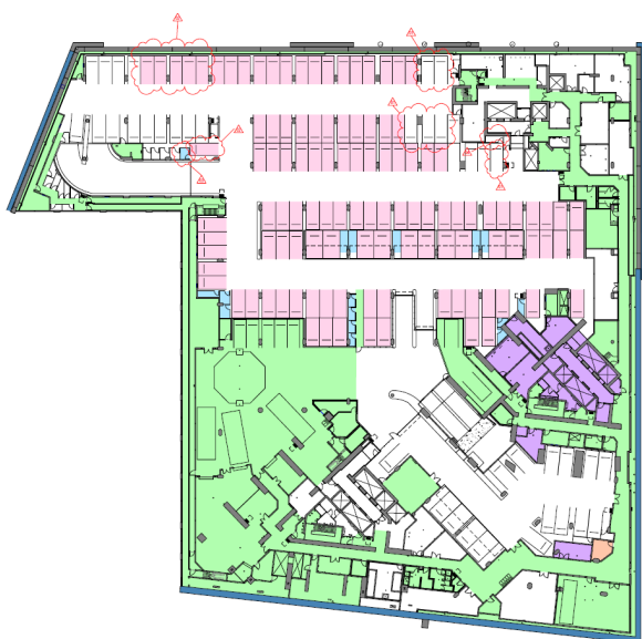
Figure 1 Proposed reallocation of parking spaces, with clouded pink spaces reallocated to Building R4B, and white, clouded spaces reallocated to R5
