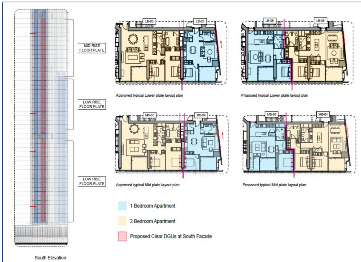
Figure 6 | Reversal of two and three-bedroom apartments LB-05 and LB-06 (levels 1-19 and 21-32) and MB-04 and MB-05 (levels 33 – 46) and revised location of DGUs (Base source: Applicant's Design Report)
