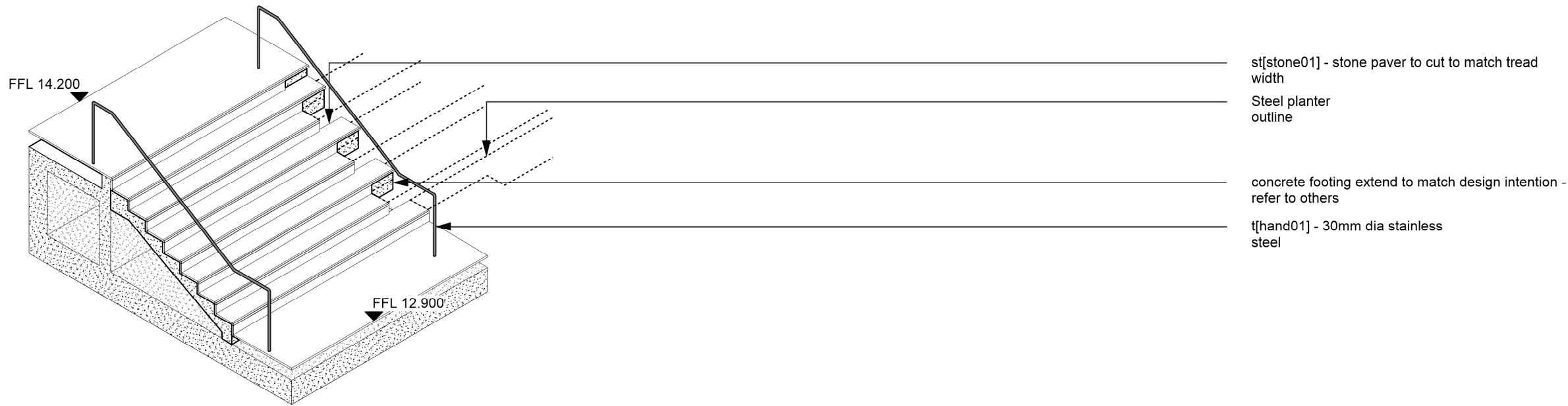
B STAIR DETAIL ISONOMETRIC - Scale 1:75
