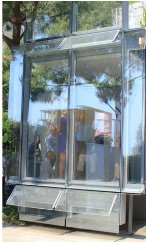
Figure 8 – An indicative full-scale mock-up of the Wintergarden facade
