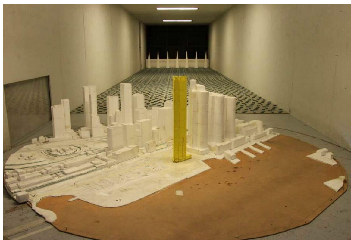
Figure 2d: Photograph of the Wind Tunnel Model (Scenario 1, view from the north-west)
