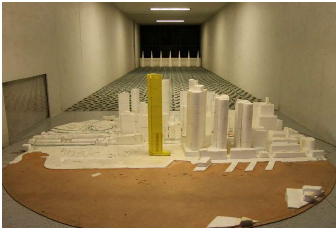
Figure 2c: Photograph of the Wind Tunnel Model (Scenario 1, view from the west)
