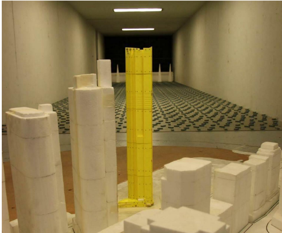
Figure 2e: Photograph of the Wind Tunnel Model (Scenario 1, view from the south-east)
