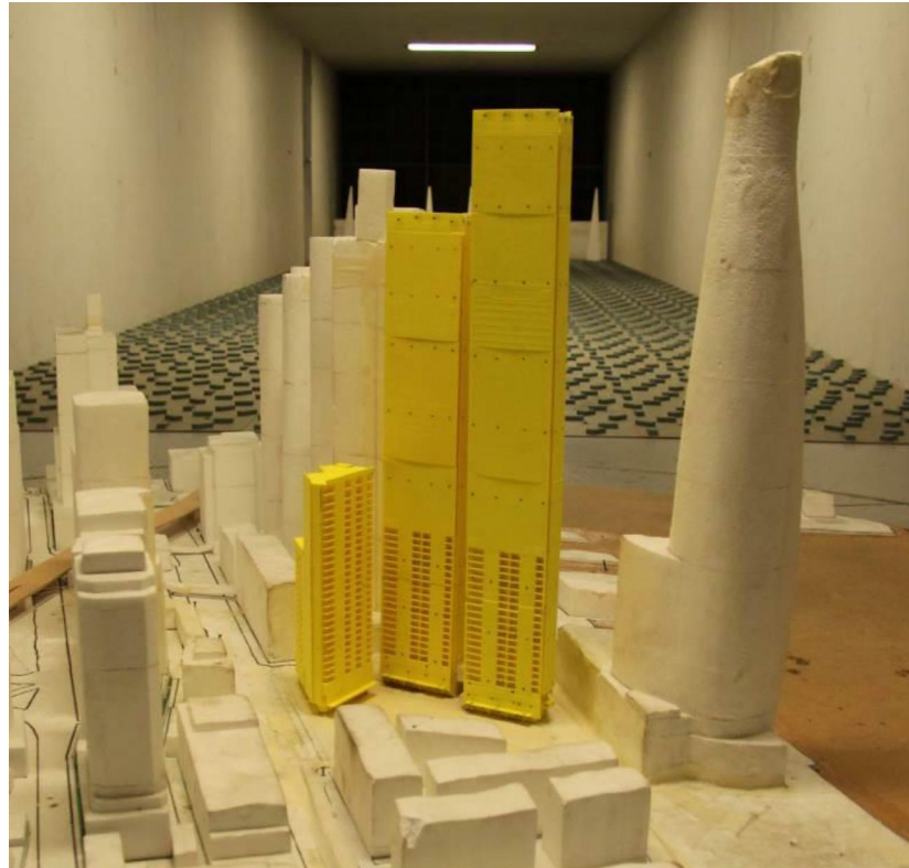
Figure 2k: Photograph of the Wind Tunnel Model (Scenario 2, view from the north)
