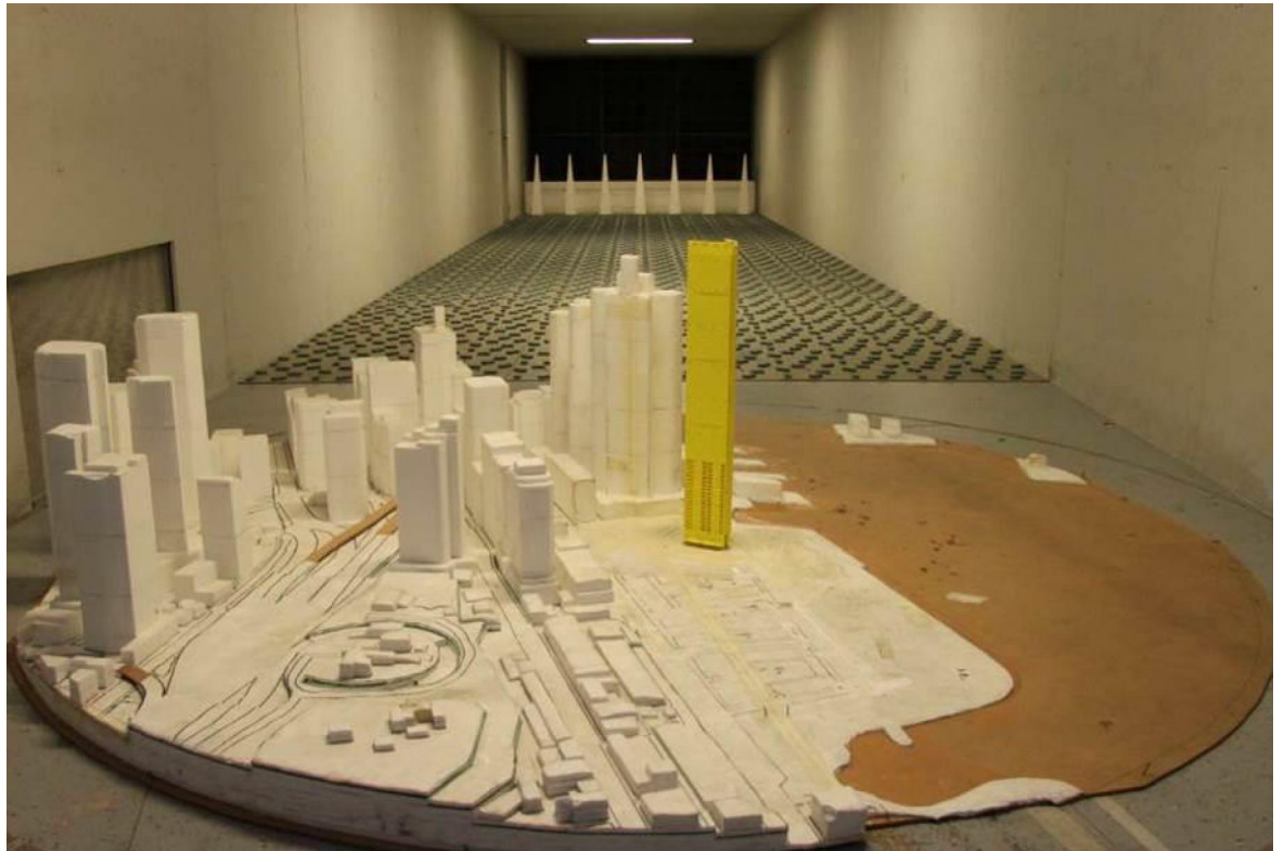
Figure 2a: Photograph of the Wind Tunnel Model (Scenario 1, view from the north)
