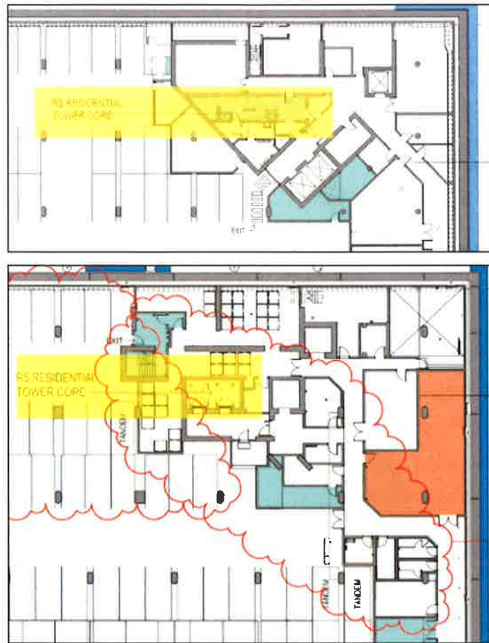
Figure 5 | The approved (above) and proposed (below) location of the Building R5 core, shown by the yellow area, on Basement Level B1 (Base Source: RPBW Architects)
