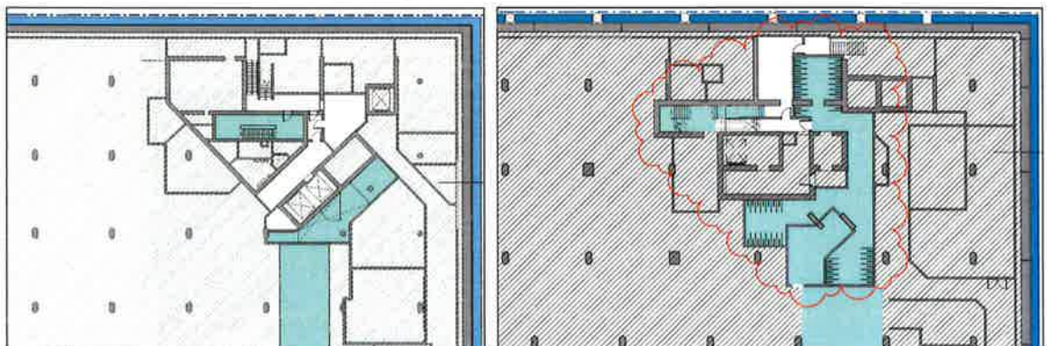
Figure 6 | The approved (left) and proposed (right) location of the Building R5 core on Basement Level B0 (Base Source: RPBW Architects)
