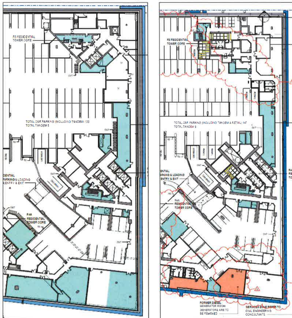
Figure 9 | The approved (left) location and proposed (right) removal of the back-up diesel generator on Level 1B shown by orange shading (Base Source: RPBW Architects)
