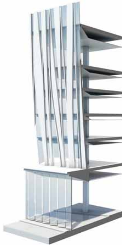
Type 2: 'Stone veil' inverse stone panel with glass infill
