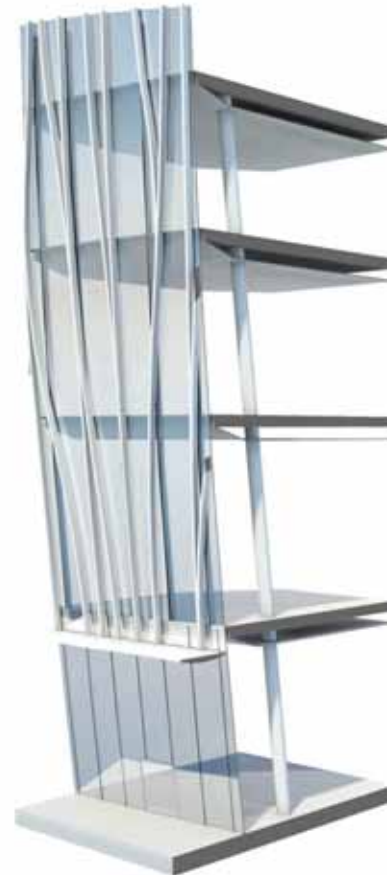
Type 3: 'Stone veil' in front of curtain wall system
