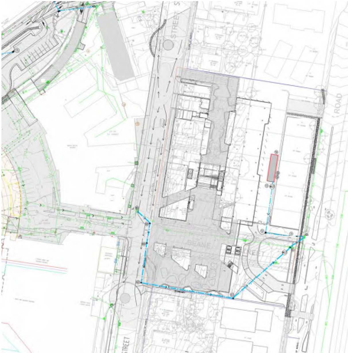
Figure 8 – Health and Well Being Precinct Stormwater System
