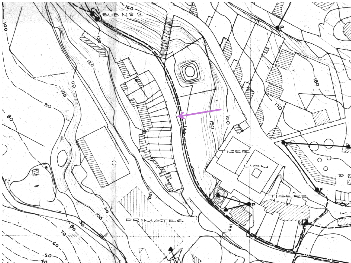
Figure 8 This detail of a Zoo plan prepared by PWD is signed by the chief engineer in 1973. It shows the high and low voltage underground electricity installation on the upper side of Dog Road. The drawing accurately shows the exhibits, ramp and lookout area on the lower side of Dog Road. Note the uneven path edge (arrowed) on the upper side. PWD plan
