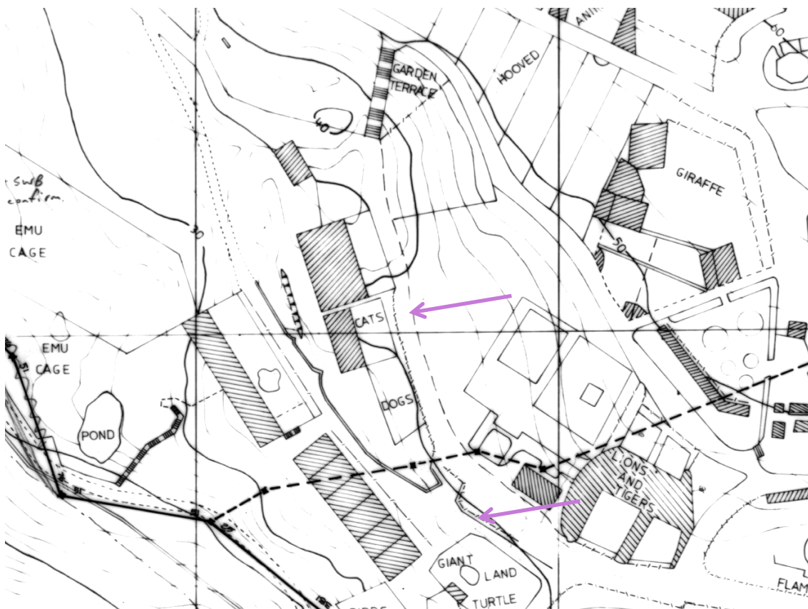
Figure 9 This PWD plan shows a main sewerage line on a survey dated 1975. The drawing does not accurately show the exhibits (eg. Tahr Mountain is missing) but shows fencing along the edge of the lookout and in front of the cat and dog exhibits. The same symbol is also used for the lions and tigers fencing. The opposite side of the road is dashed (not kerbed??). PWD plan
