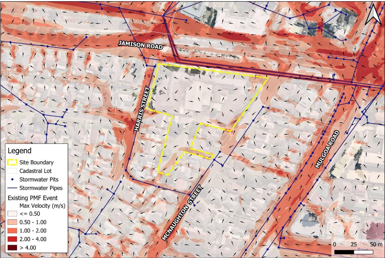
Figure 14: PMF velocities at the site under existing conditions
