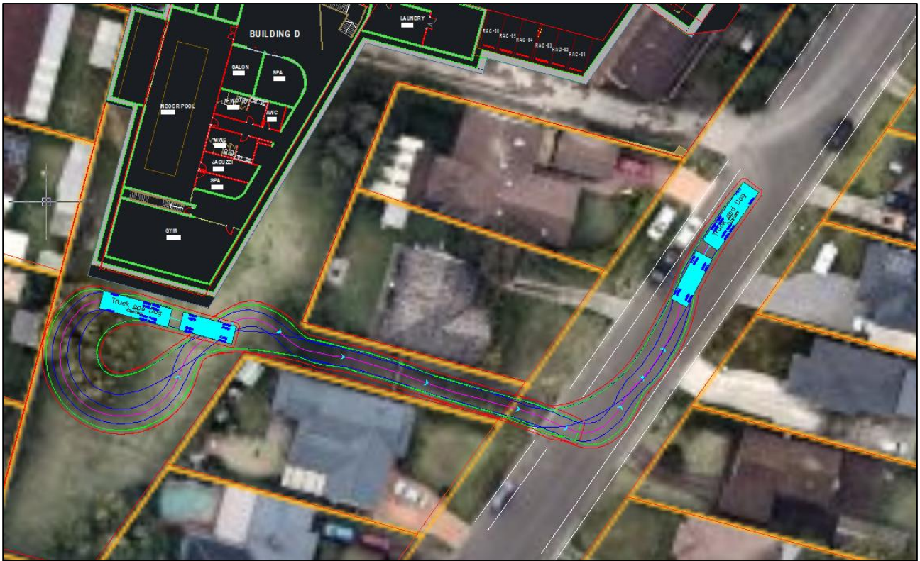
EXCAVATION PHASE – TRUCK AND DOG FORWARD EXIT (OPTION ONE)
