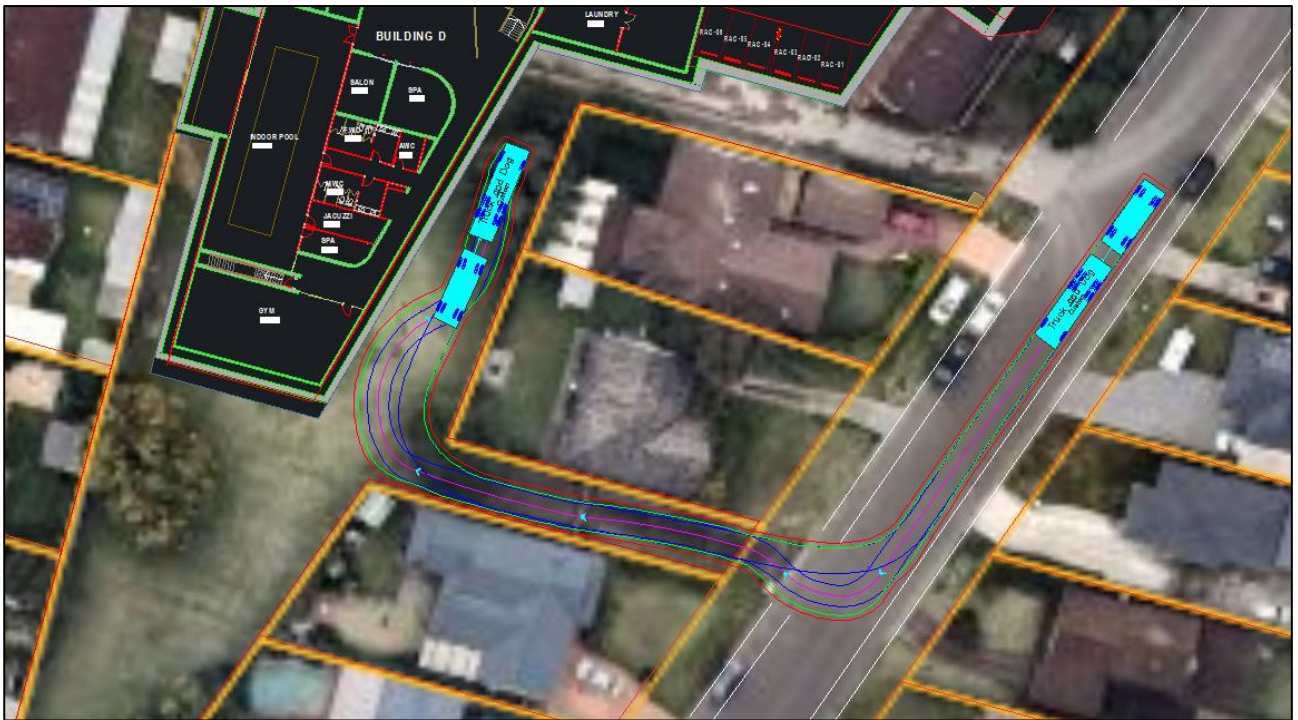
EXCAVATION PHASE – TRUCK AND DOG FORWARD ENTRY (OPTION TWO)
