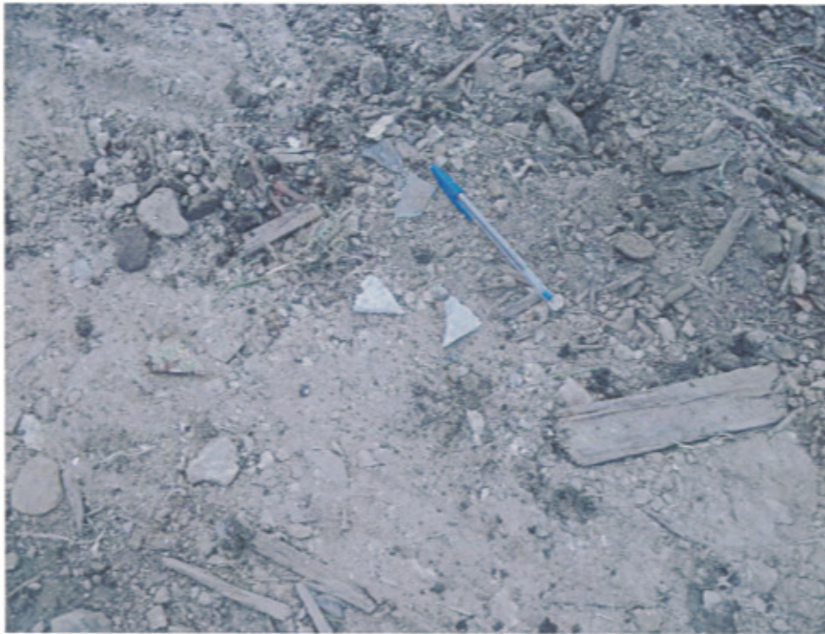
Photograph 21: Possible ACM fragments on the ground surface of 26 Dalziell Street
