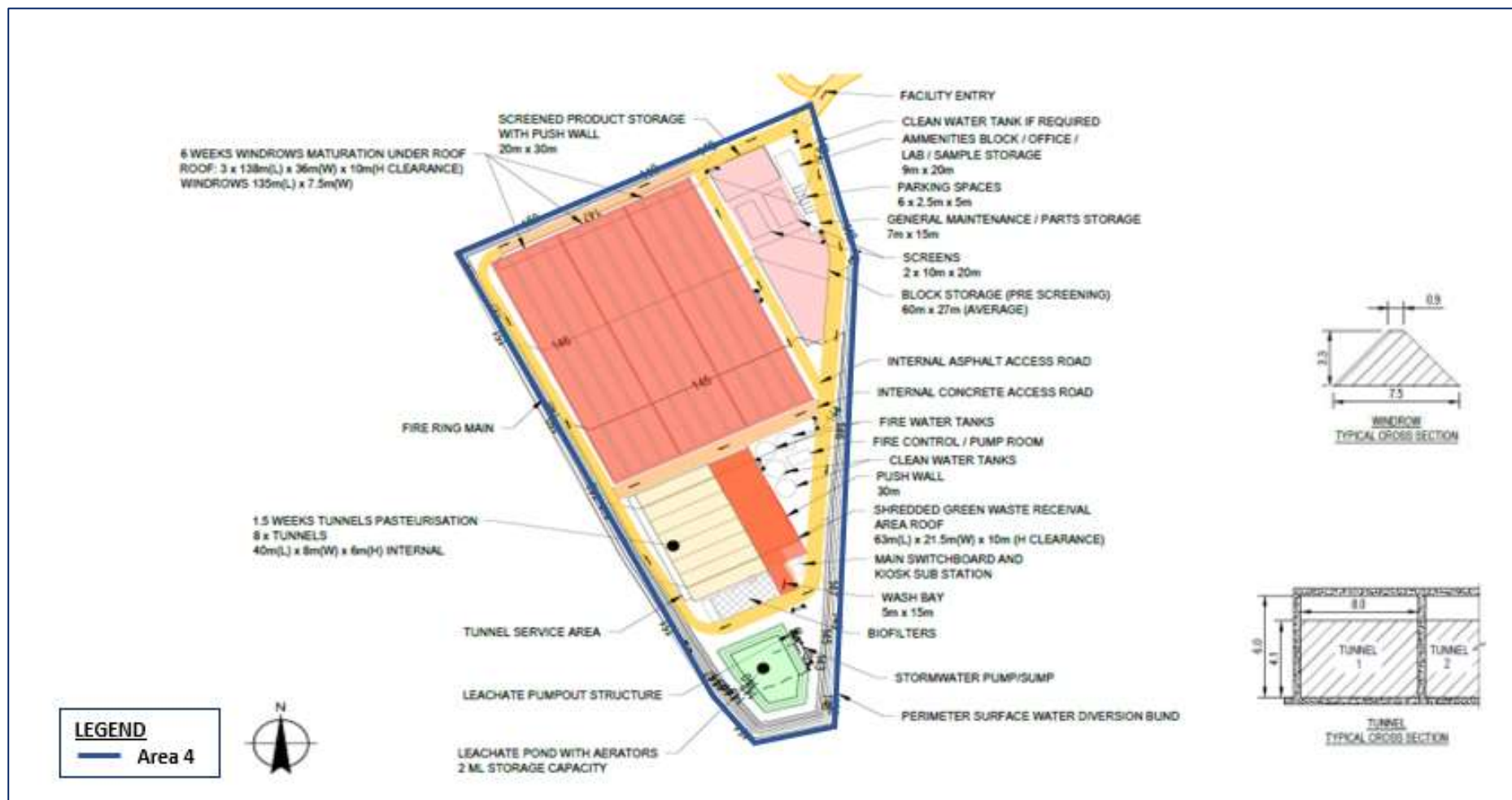
Figure 4: Garden Organics Facility – western GO operational area
