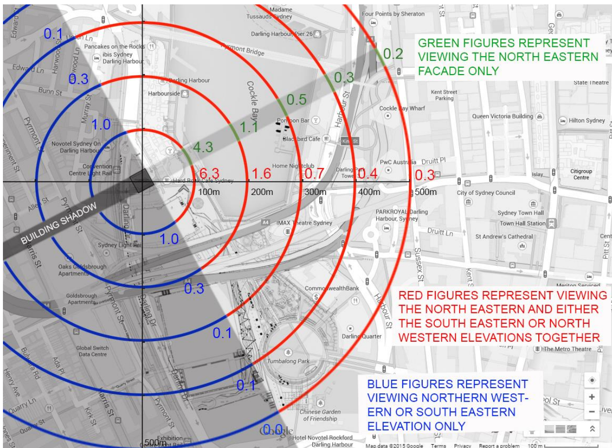
Figure 6 Theoretical illuminance contour diagram
