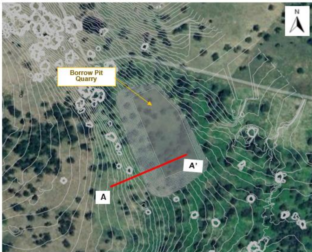
Figure 5 Plan View of Proposed 'Borrow Pit' at Liverpool Range Quarry Depicting Nominated Stability Section
