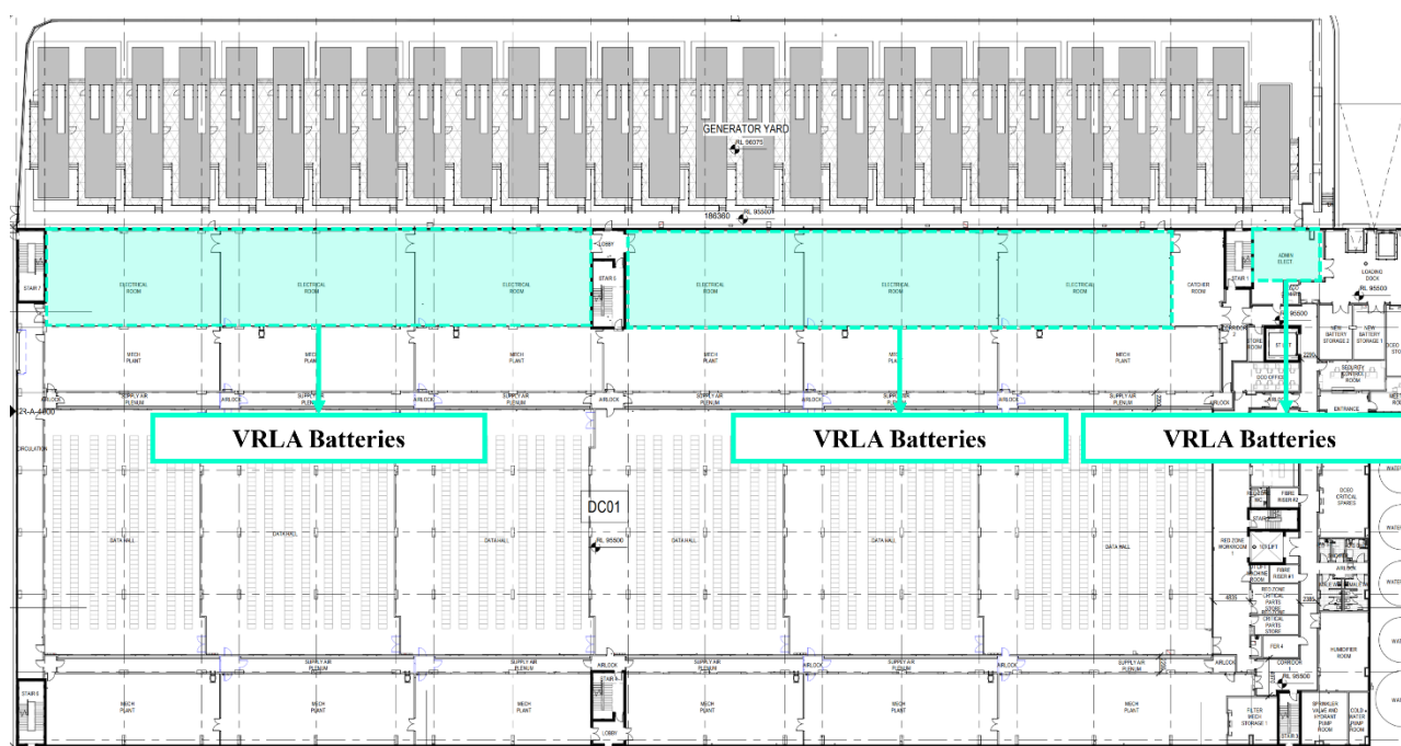
Figure 2-8: Location of VRLA batteries on ground floor.
