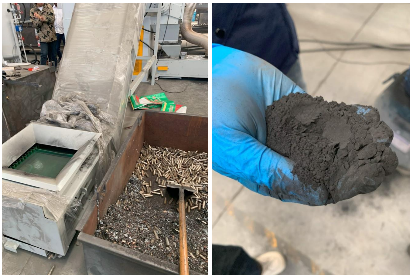
Figure 6-14 Feedstock at the feed conveyor and the black mass powder produced by the recycling process
