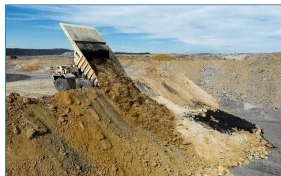
Plate 3: In-pit Waste Rock Emplacement by Haul Truck
