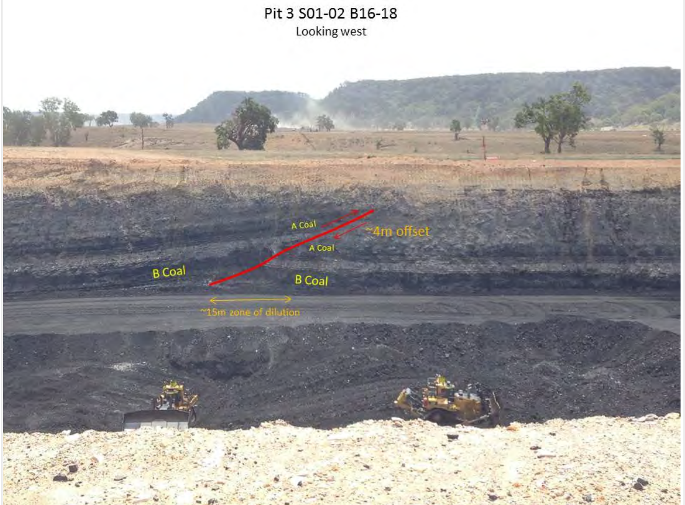
Photo in centre of Pit 3, looking west. Shows fault intersected in this pit.
