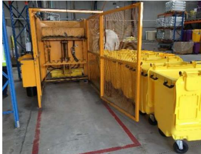
Figure 9 | Bin Lifter at the Facility
