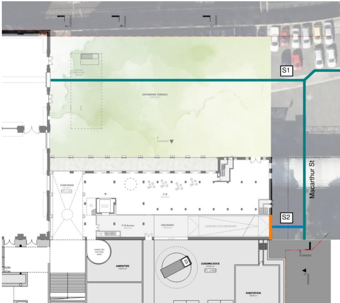
Figure 12 - Modelled loading routes. Medium truck path shown in BLUE, Large truck path shown in GREEN. Extent of loading dock door shown in ORANGE
