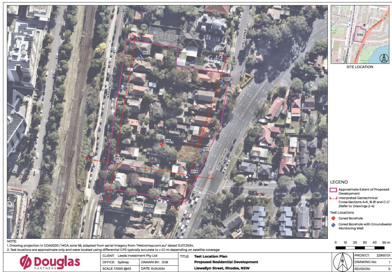
Figure 15 – Borehole Location Plan Source: Douglas Partners, September 2024. Drawing No. 1.
