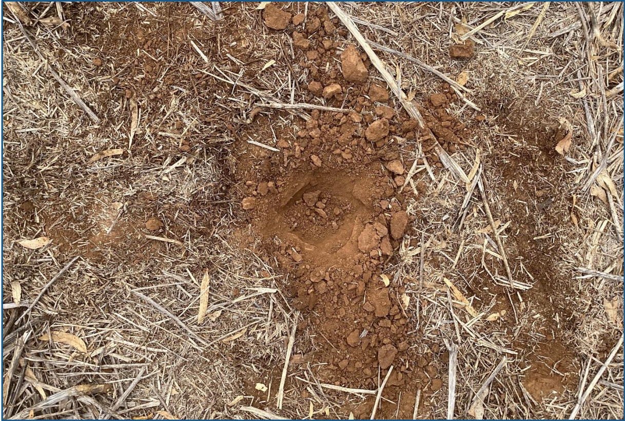
Image 2: A sample of surface soil was collected from the site with a decontaminated 100mm diameter hand auger.
