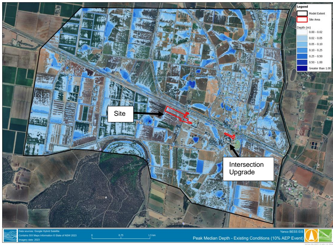
Figure B 1 Existing Conditions – 10% AEP flood depth
