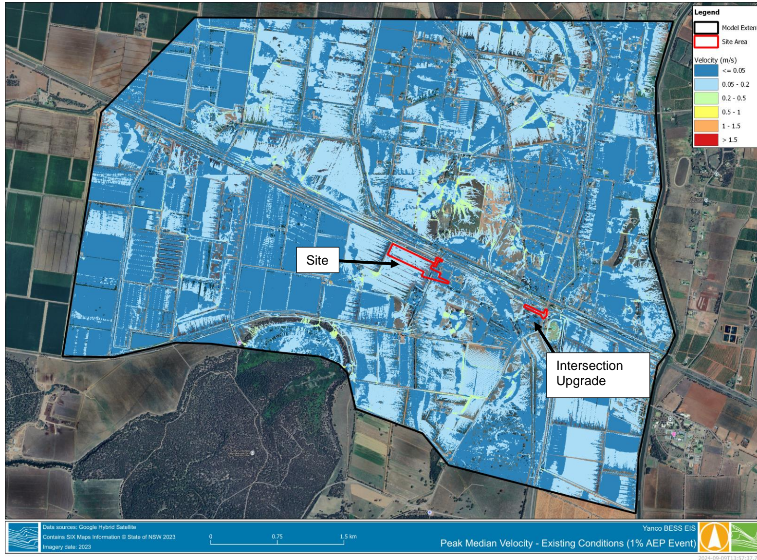
Figure 5-5 Existing Conditions – 1% AEP flood velocity
