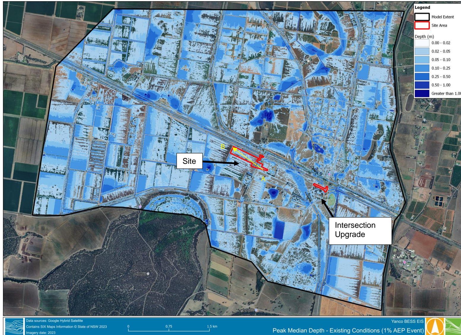
Figure 5-3 Existing Conditions – 1% AEP flood depth
