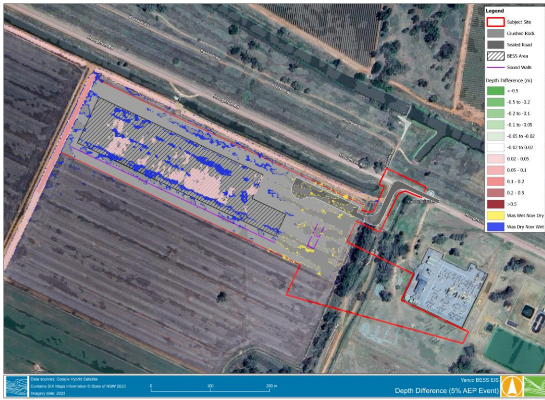
Figure C 3 Design Conditions – 5% AEP flood depth
