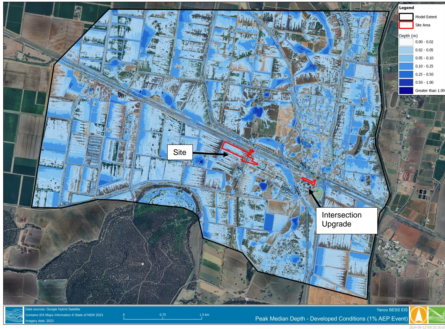
Figure 5-9 Developed Conditions – 1% AEP flood depth
