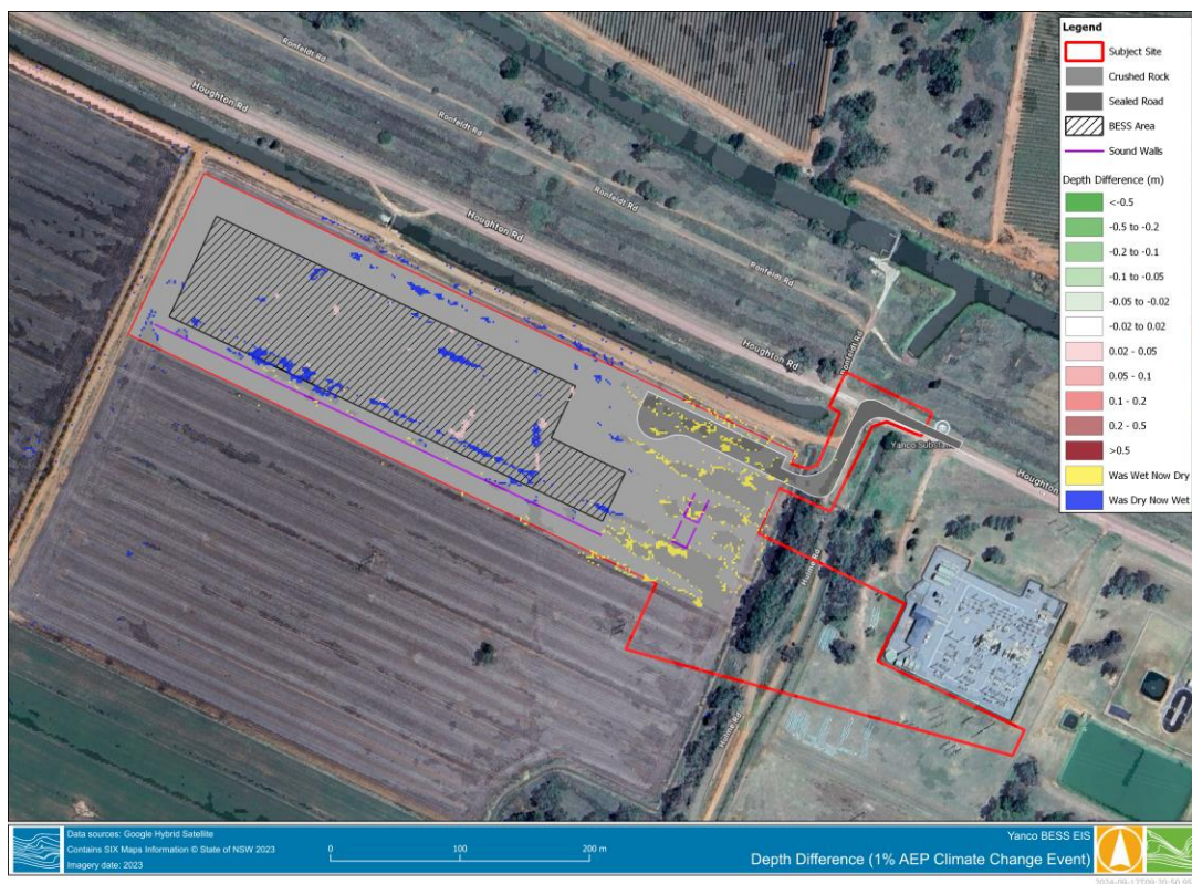
Figure C 5 Design Conditions – 1% AEP + Climate Change flood depth
