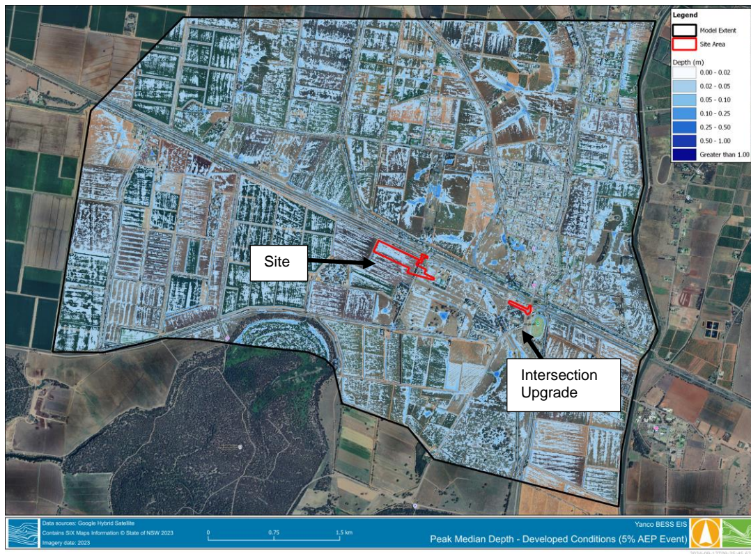
Figure C 3 Design Conditions – 5% AEP flood depth
