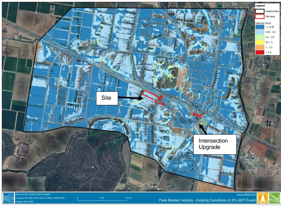
Figure B 11 Existing Conditions – 0.5% flood velocity
