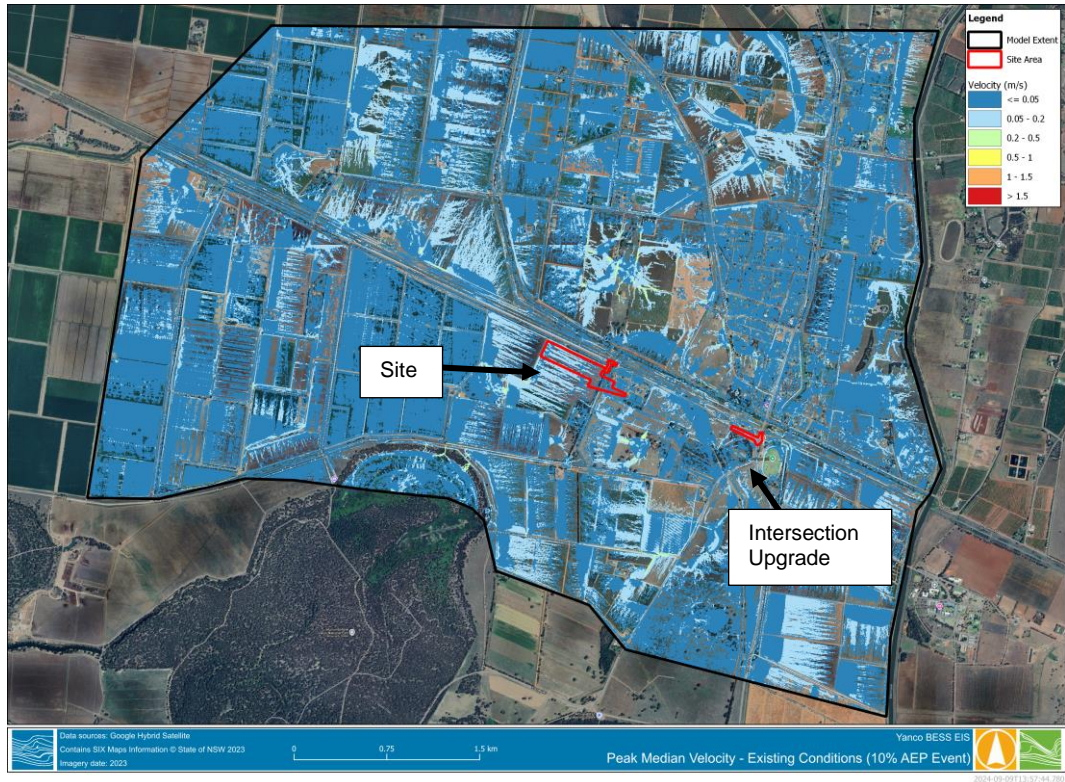
Figure B 2 Existing Conditions – 10% AEP flood velocity
