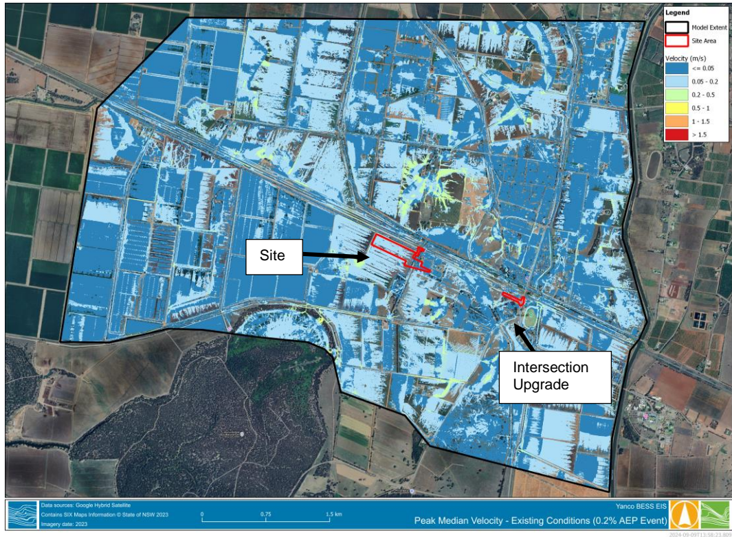
Figure B 14 Existing Conditions – 0.2% flood velocity
