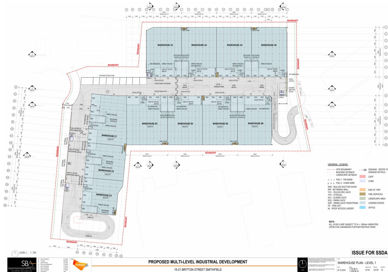
Figure 3-4: Level 1 Warehouse Layout
