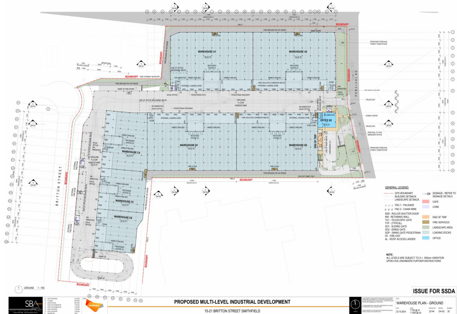
Figure 3-3:Ground Level Warehouse Layout
