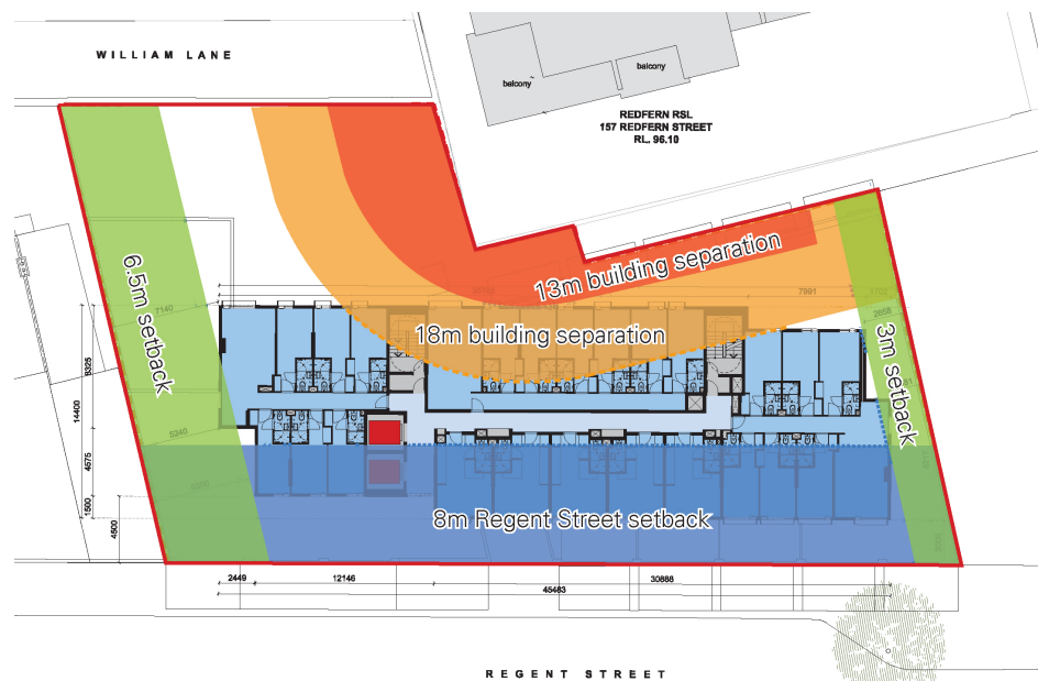
Figure 7 – Diagrams illustrating setbacks required under the Draft Urban Design Guidelines for Redfern Source: Bates Smart
