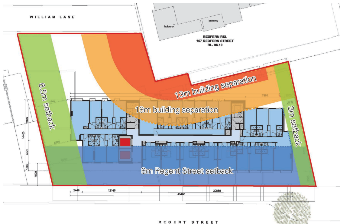
Figure 18 – Diagram illustrating setbacks required under the Draft Urban Design Guidelines for Redfern
