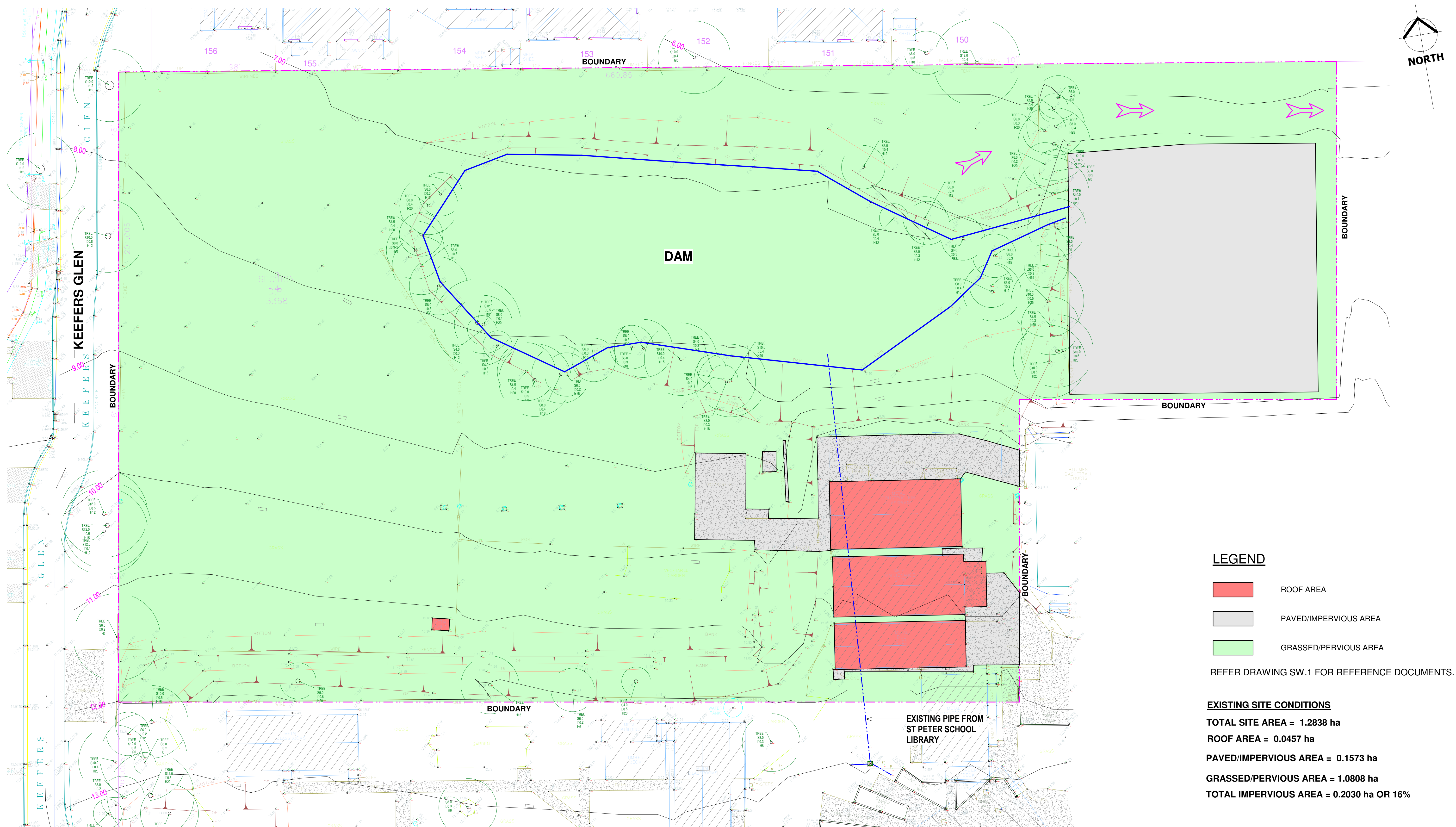
STORMWATER CATCHMENT PLAN - EXISTING SITE
