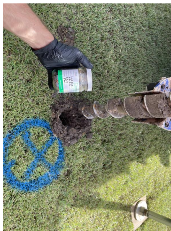
Photo 4: Sample S06_0.6 next to the drill rig. No stains or odours noted.
