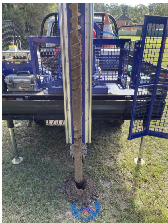
Photo 3: Advancement of BH01. No stains or odours noted.
