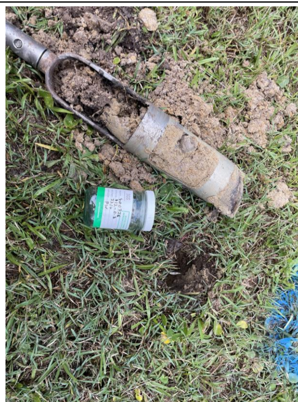
Photo 6: Sample S12_0.3. No stains or odours noted.
