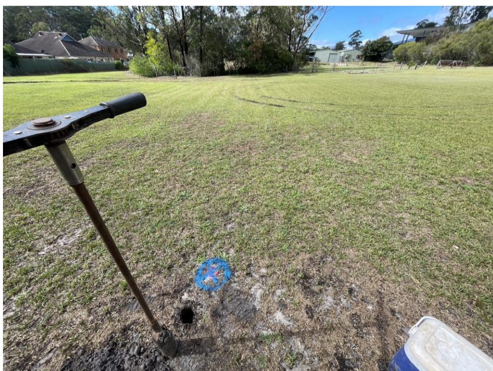
Photo 5: BH03 being drilled using a hand auger. No stains or odours noted.
