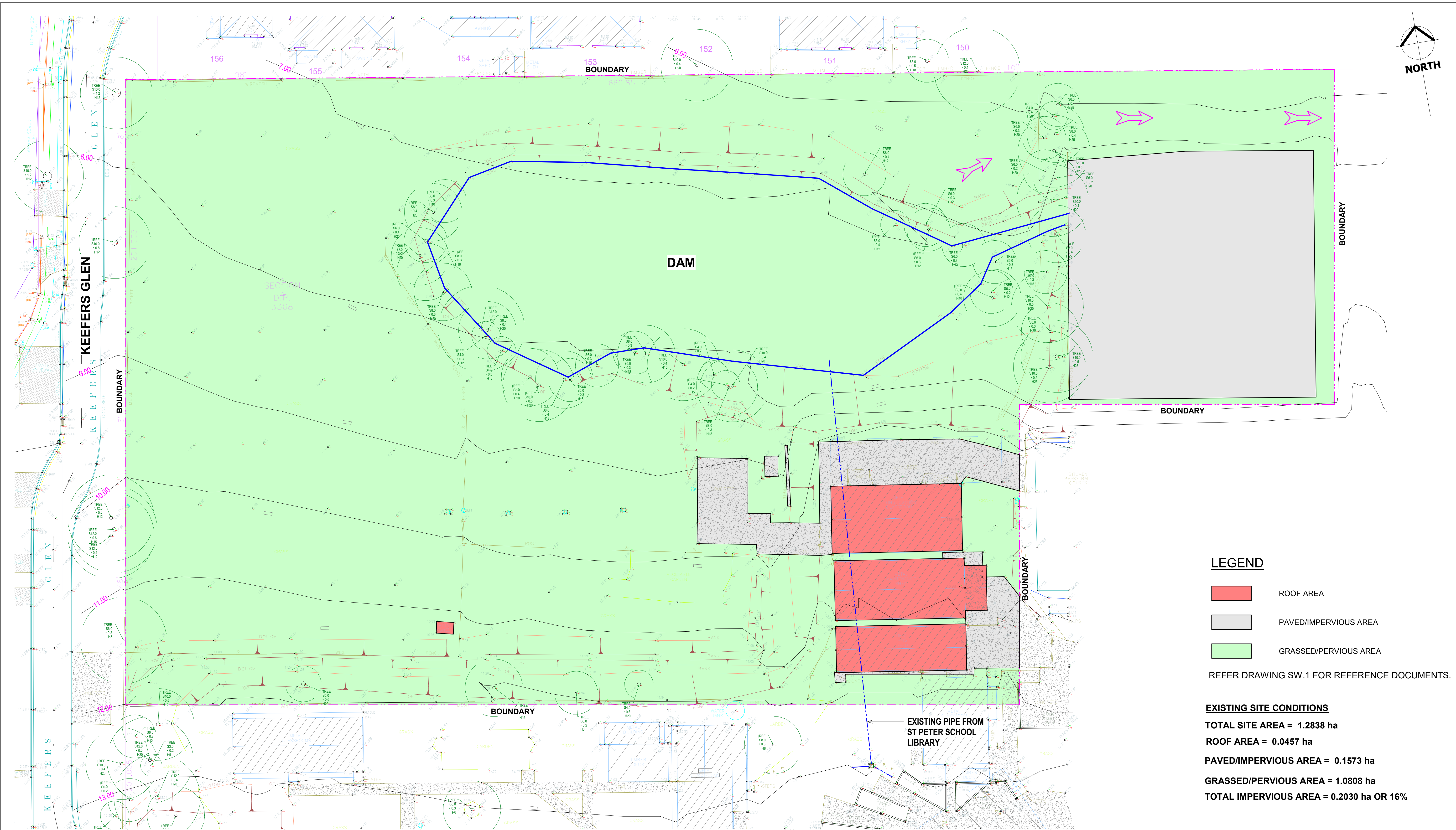
STORMWATER CATCHMENT PLAN - EXISTING SITE SCALE1 : 250 @A1
