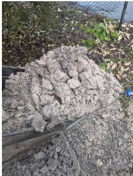
Photo 4: Image showing excavator advancing test pit excavation sample location “S20”. While fill material was noted in this sample location, material sampled still meets the ENM criteria for classification. No asbestos detected.
