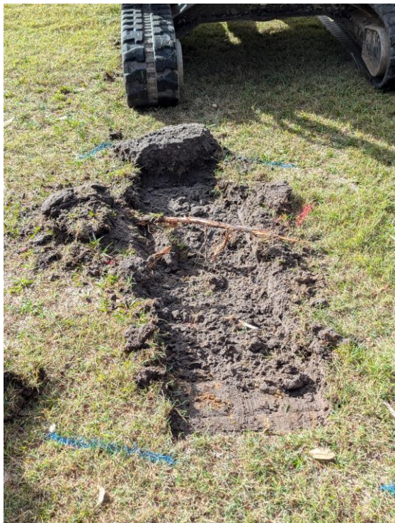
Photo 1: Image showing natural sands situated beneath grass layer. Much of the soils profiles on site were noted to be consistent with this.
