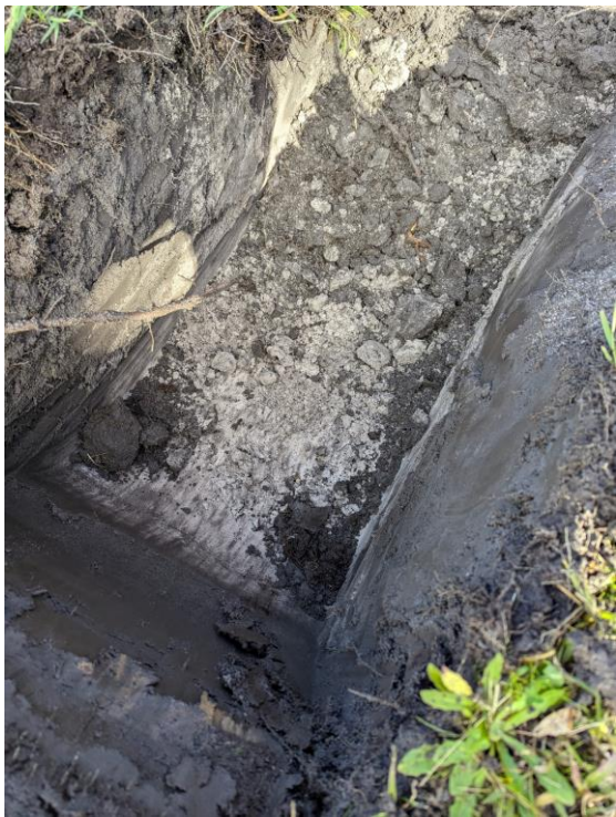
Photo 2: Deeper test pit excavation location at location “S1”. Natural sands encountered.
