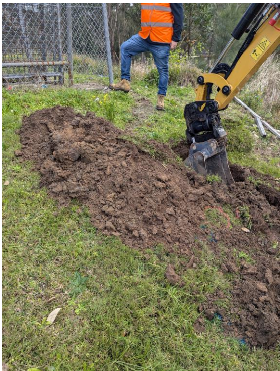
Photo 4: Image showing excavator advancing test pit excavation sample location “S20”. While fill material was noted in this sample location, material sampled still meets the ENM criteria for classification. No asbestos detected.
