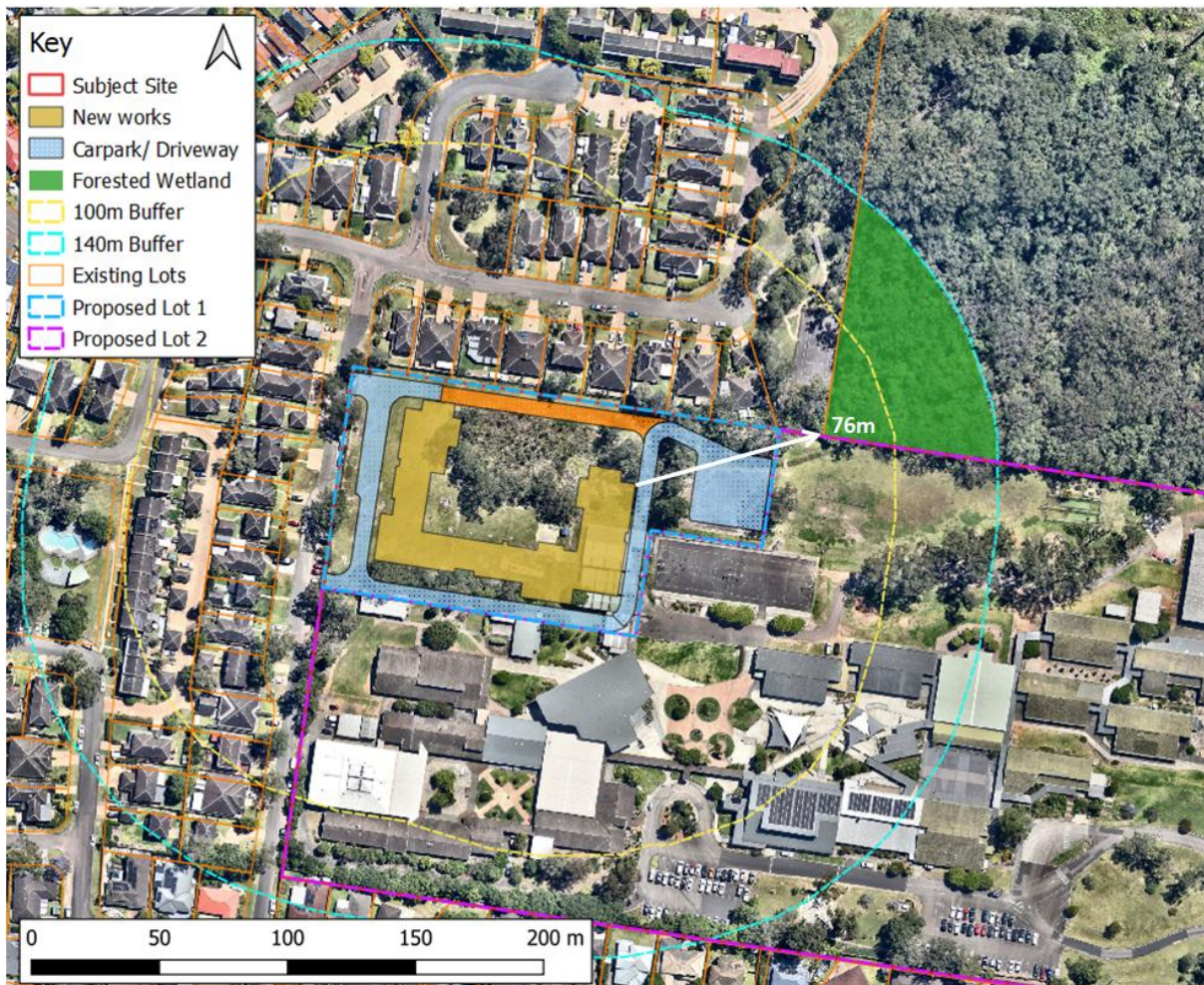
Figure 5. Hazardous vegetation affecting the subject building. Source: NearMap (2023) with overlays by BFCS P/L
