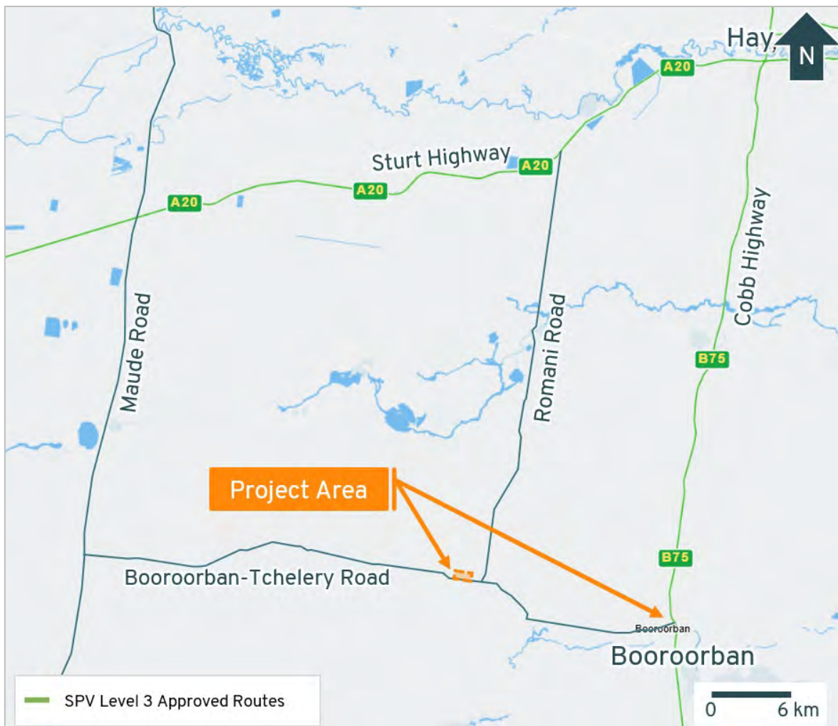
Figure 12: NHVR SPV Level 3 Network Approved Roads
