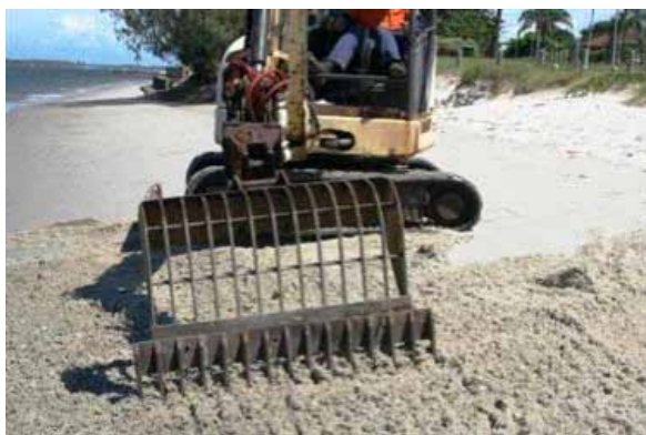
Figure 8.3. Small excavators with screening buckets deployed on beach areas
