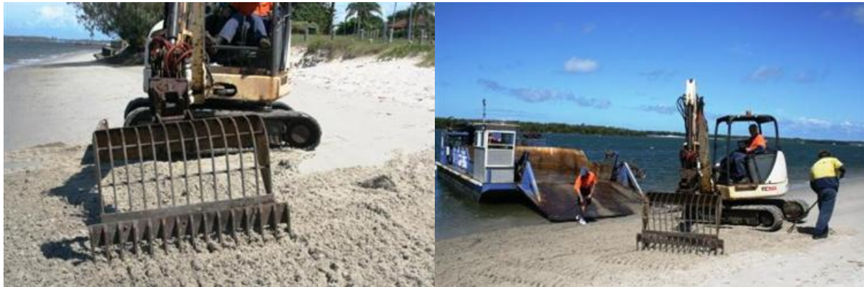
Figure 23: Small excavators with screening buckets deployed on beach areas
