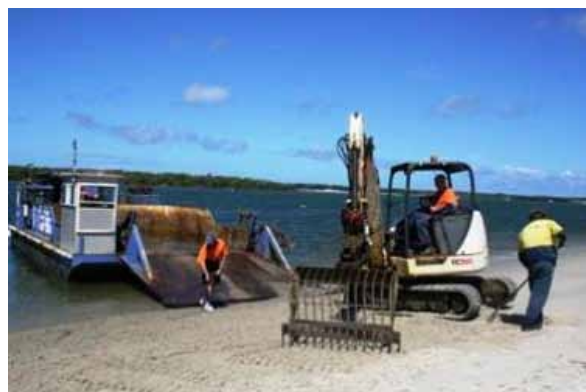
Figure 8.3. Small excavators with screening buckets deployed on beach areas
