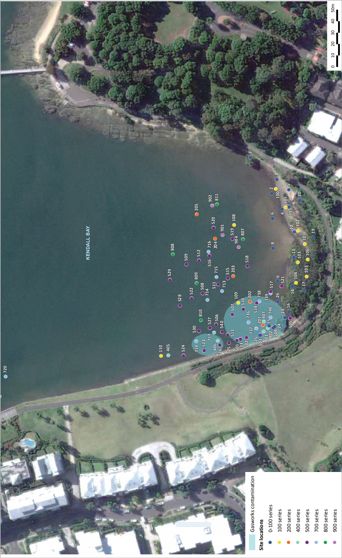
Figure 5.7. Areas where gasworks contamination is found in surface sediment – Southern Investigation Area
