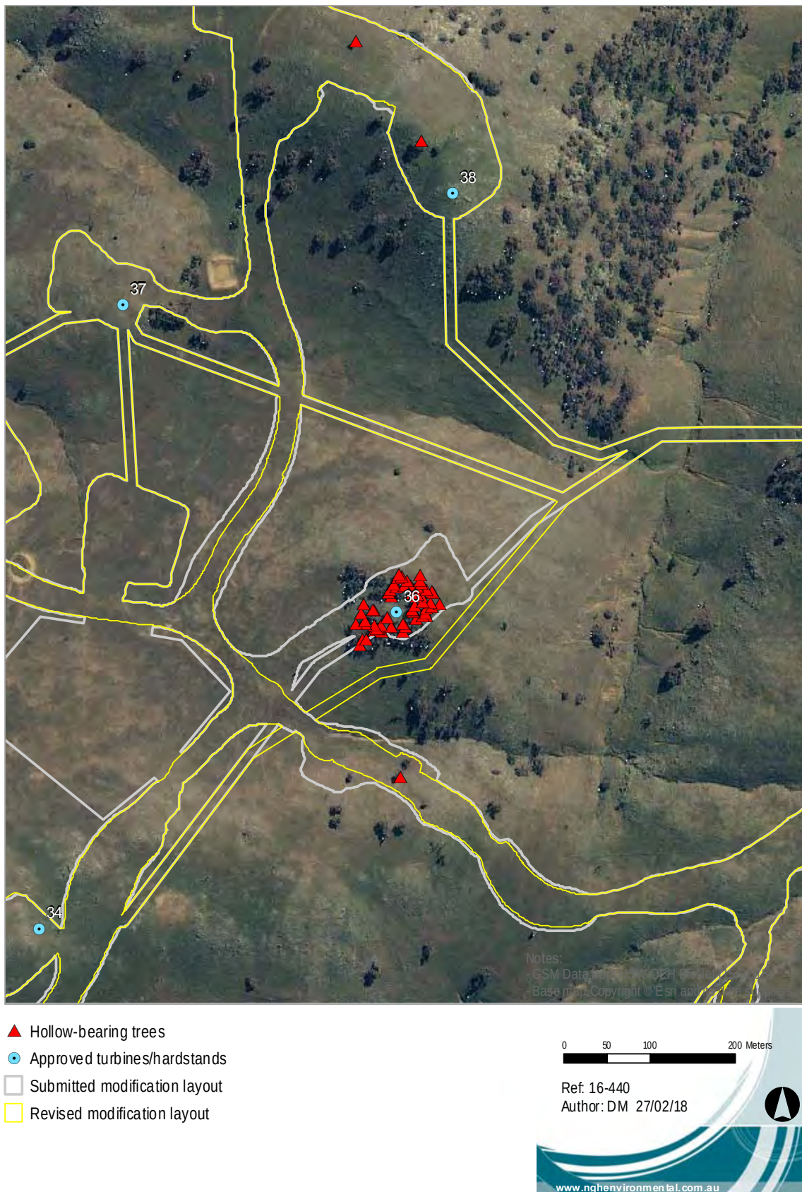
Figure 5-1 HBTs to be avoided by removing Turbine 36
