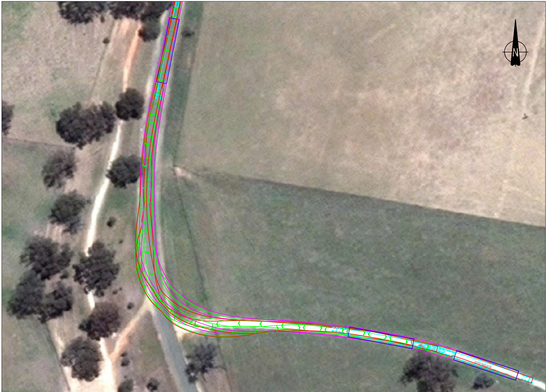
Illalong Road - Mariba West Site Access. Nootboom Tower Trailer
