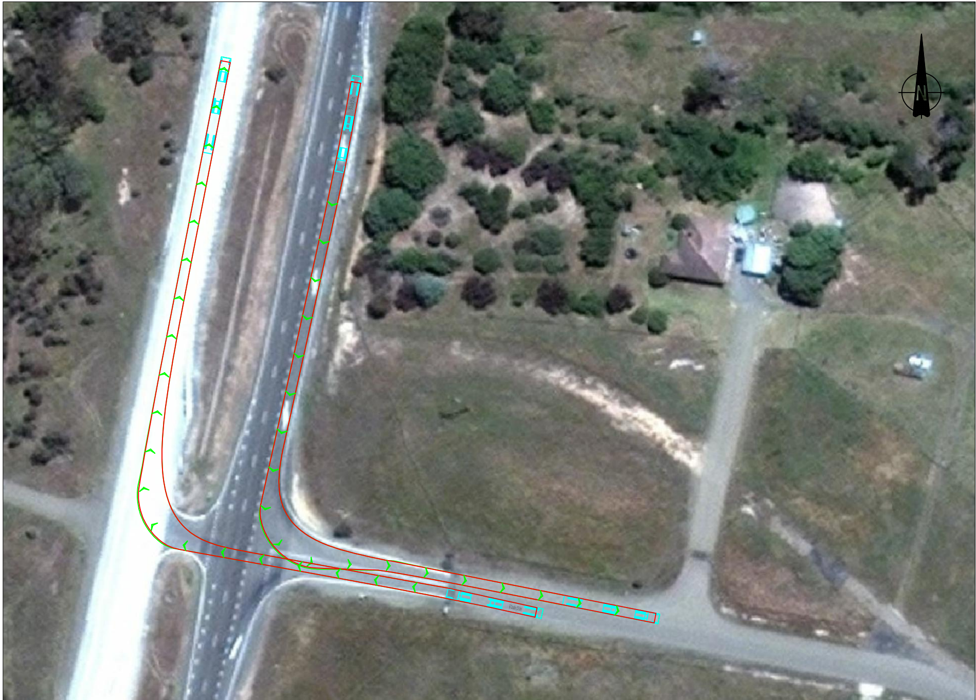
Hume Highway - Paynes Road. B-Double (25m)
