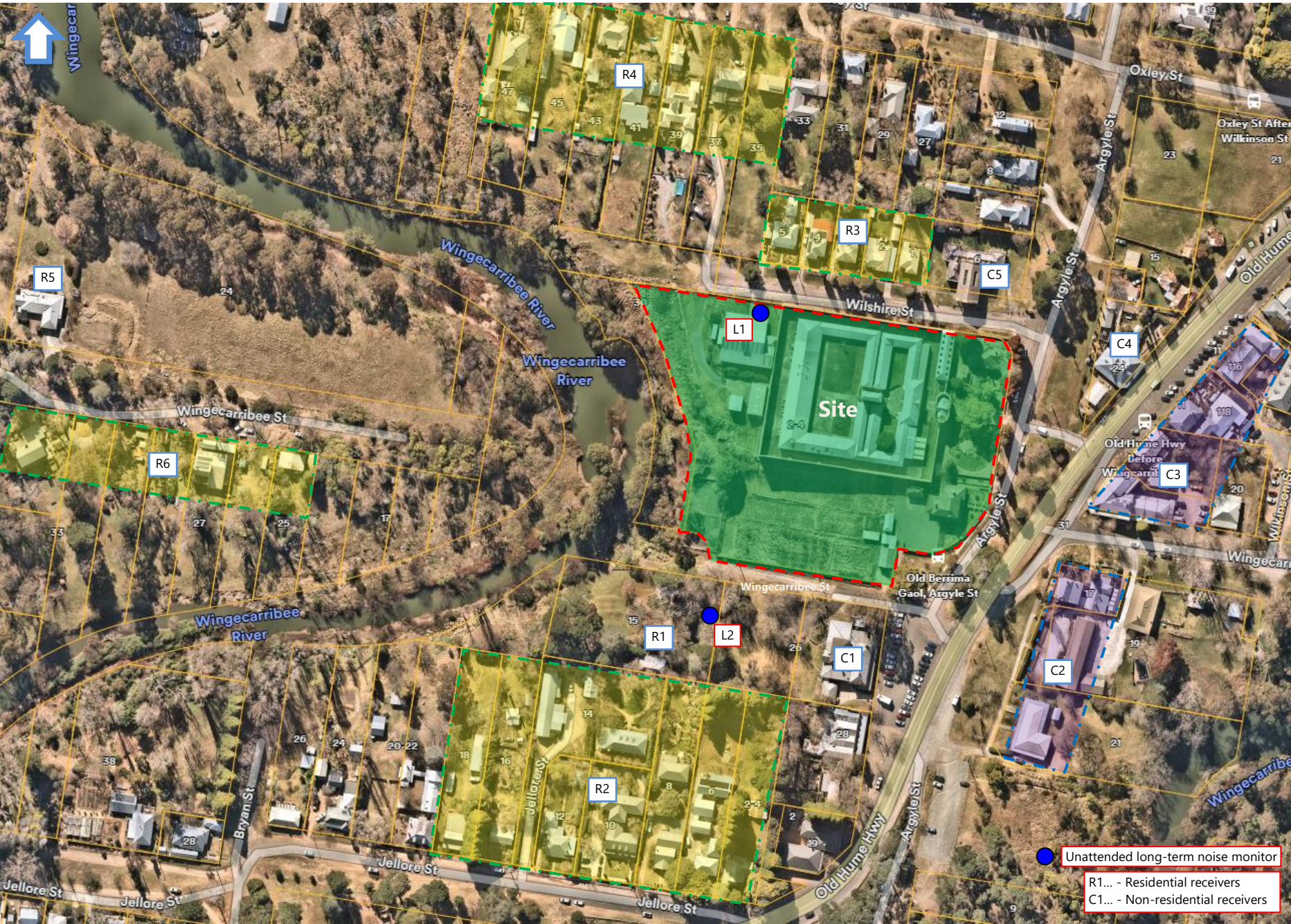
Figure 2-2: Noise Monitoring Locations and Site Surrounds
