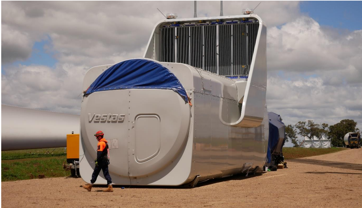
Figure 4-9: Example of a nacelle for a 3.6 MW WTG at Sapphire Wind Farm
