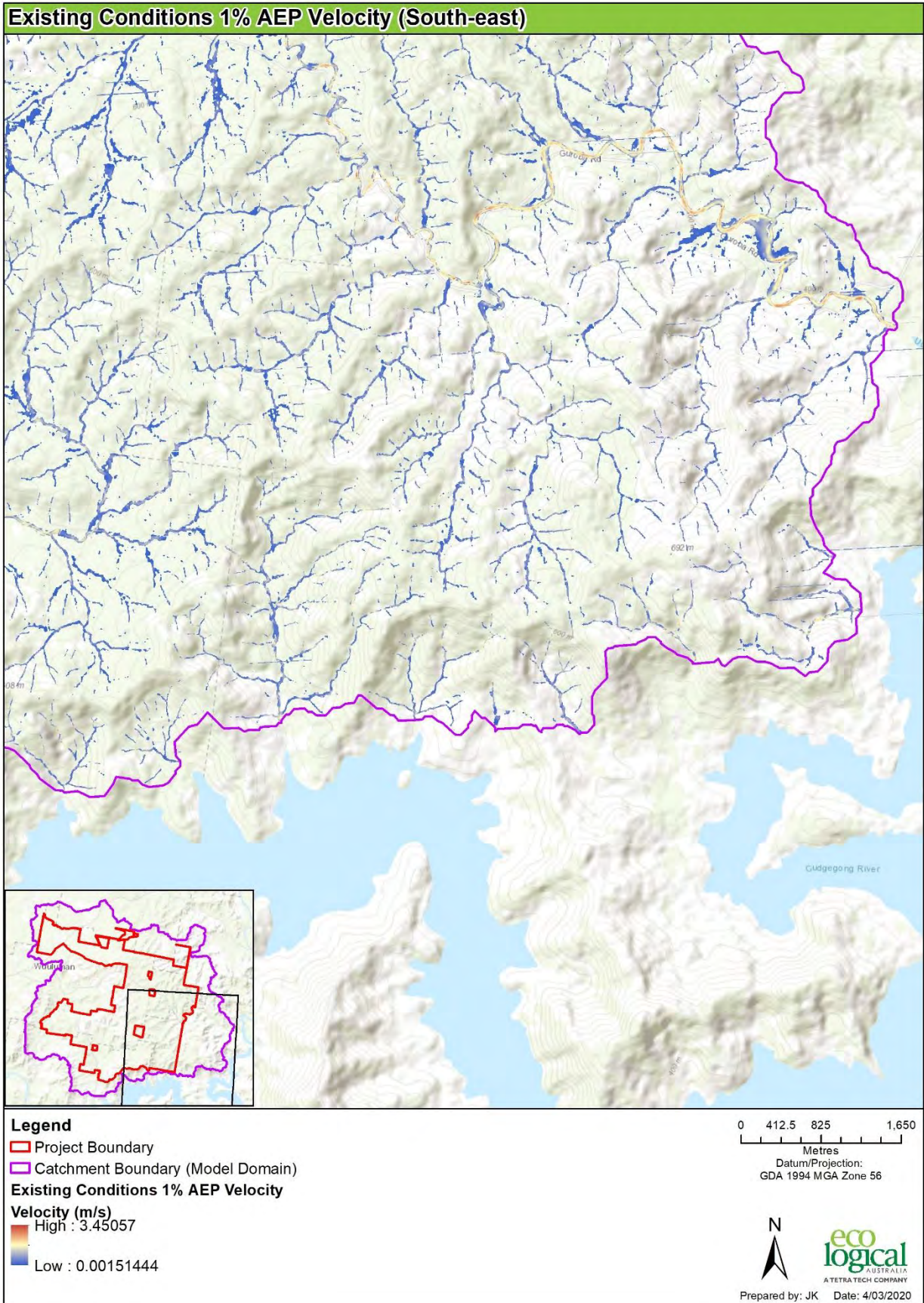
Figure 6-28 1% AEP Existing Conditions Velocities - South East
