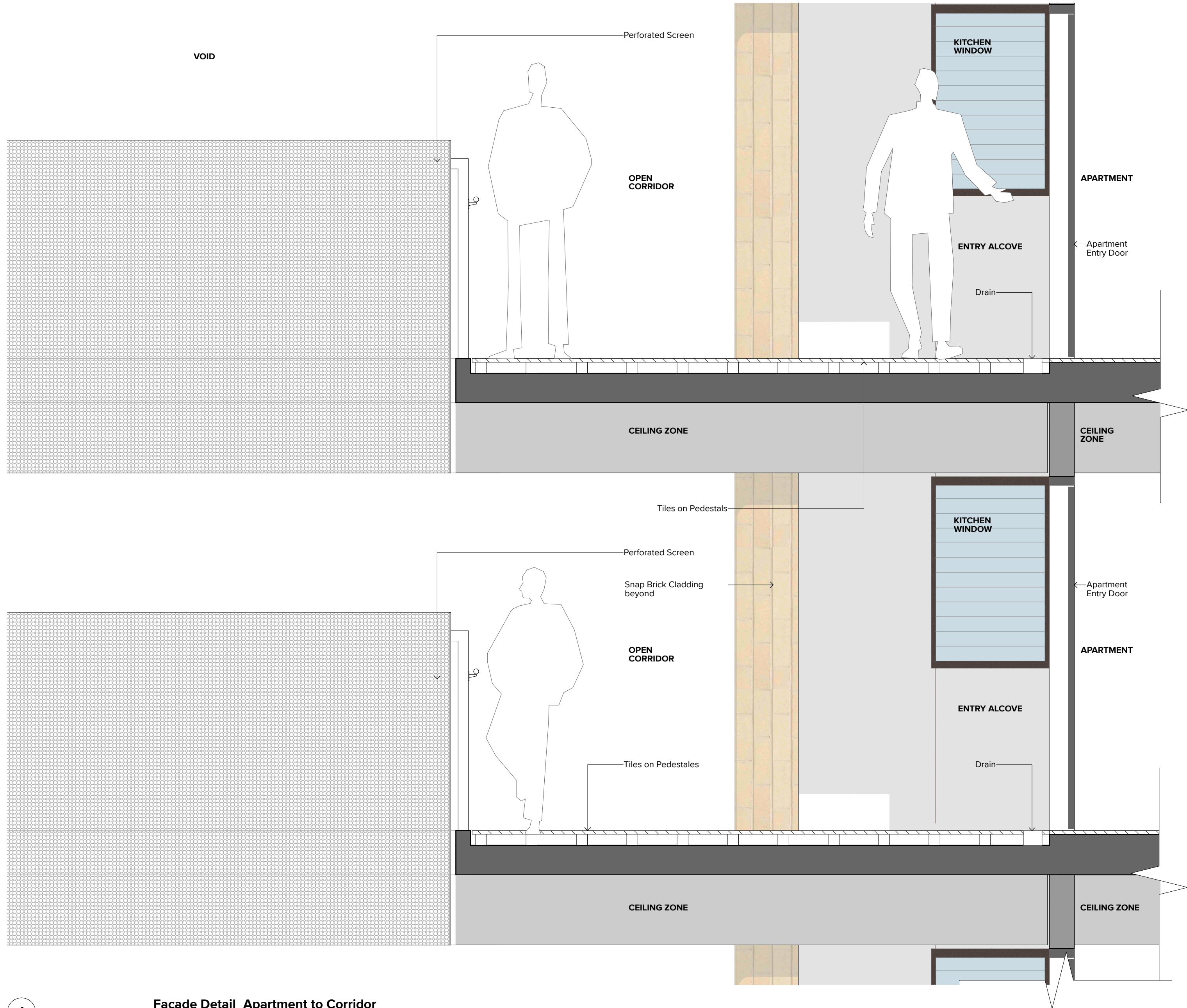
1 Facade Detail_Apartment to Corridor 1:20
