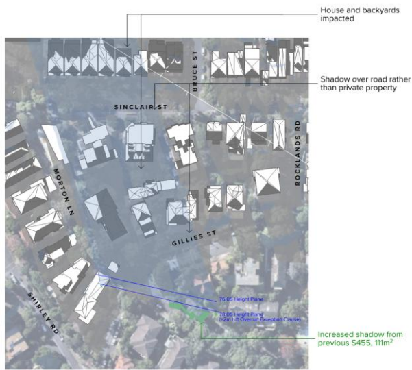
Figure 3 Additional Shadows at 9AM (Source: Turner)
