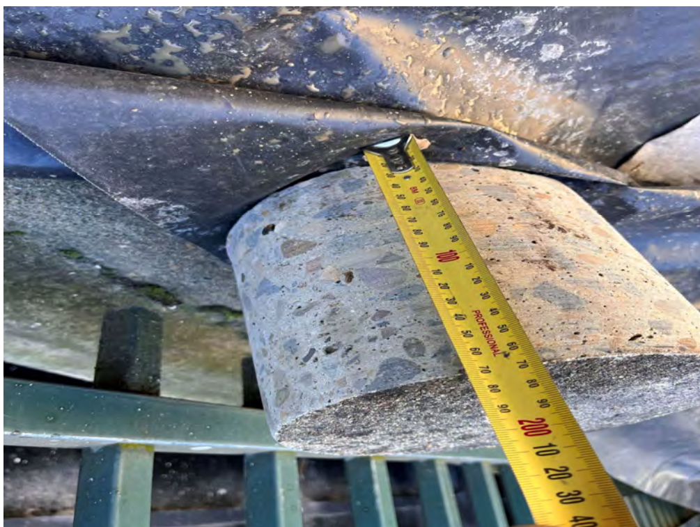
Photo 14 - Measurement of the Depth of Concrete Core at BH10
