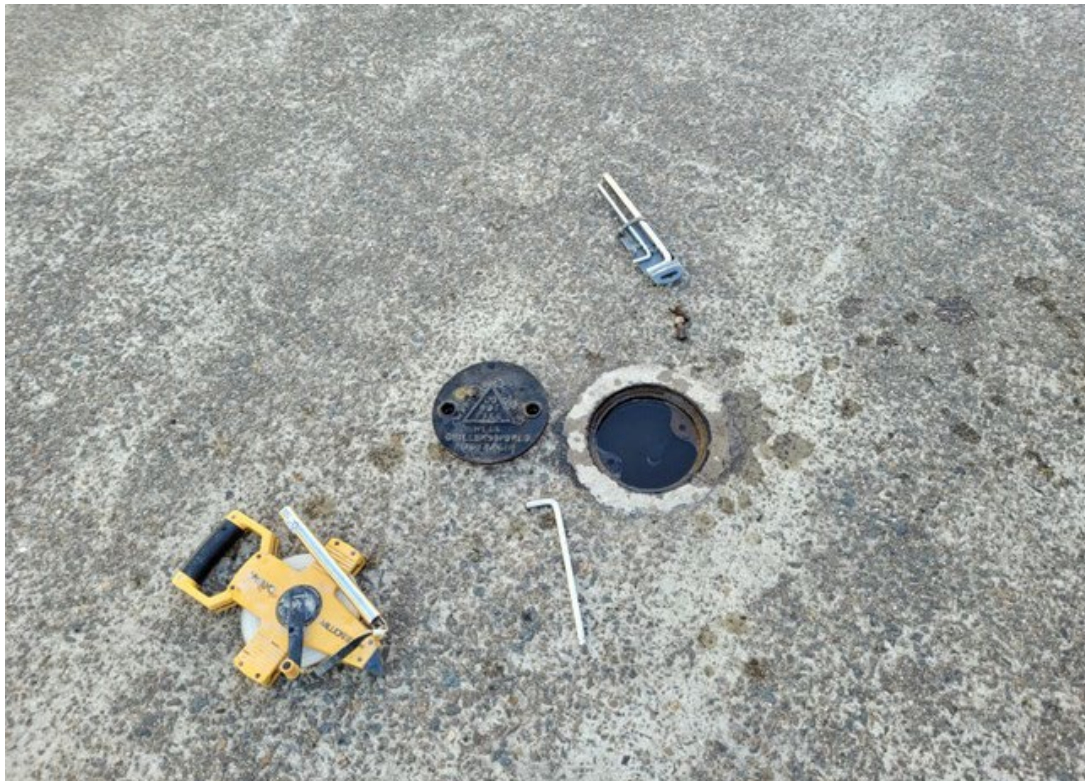
Photo 3 - Water observed outside of well casing at BH12 prior to removal of PVC cap (26 July 2023)
