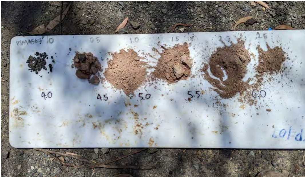
Photo 6 - Soil profile at BH04
