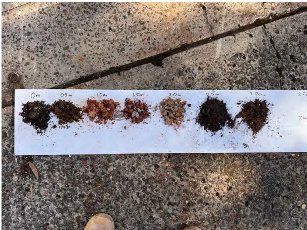
Photo 15 - Soil Profile at BH11
