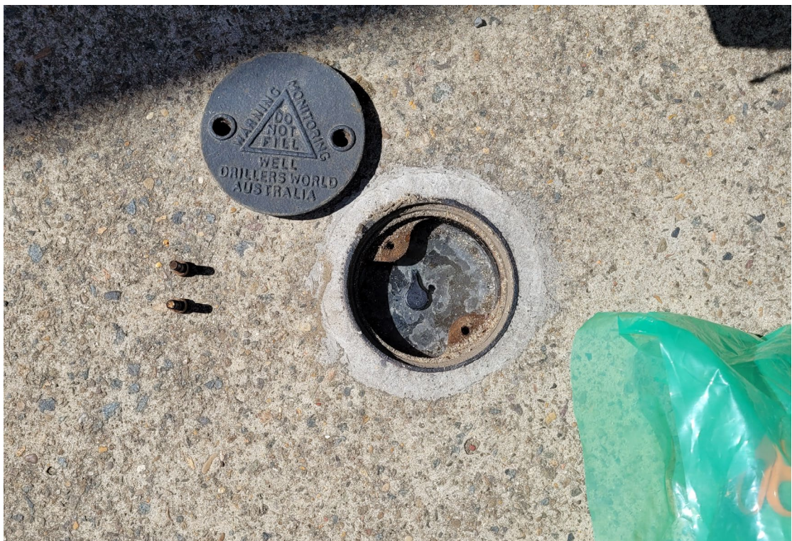
Photo 1 - Water observed outside well casing of BH1 on 18 November 2022
