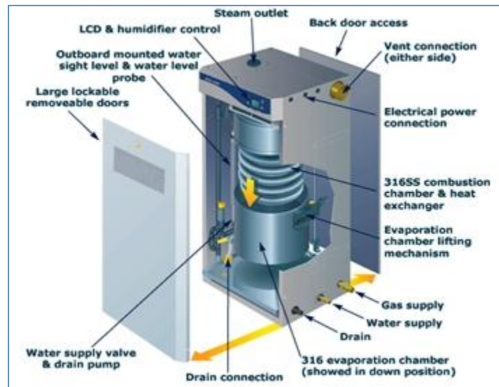
Figure 2 – Gas Humidifier (Picture courtesy of JS Humidification)
