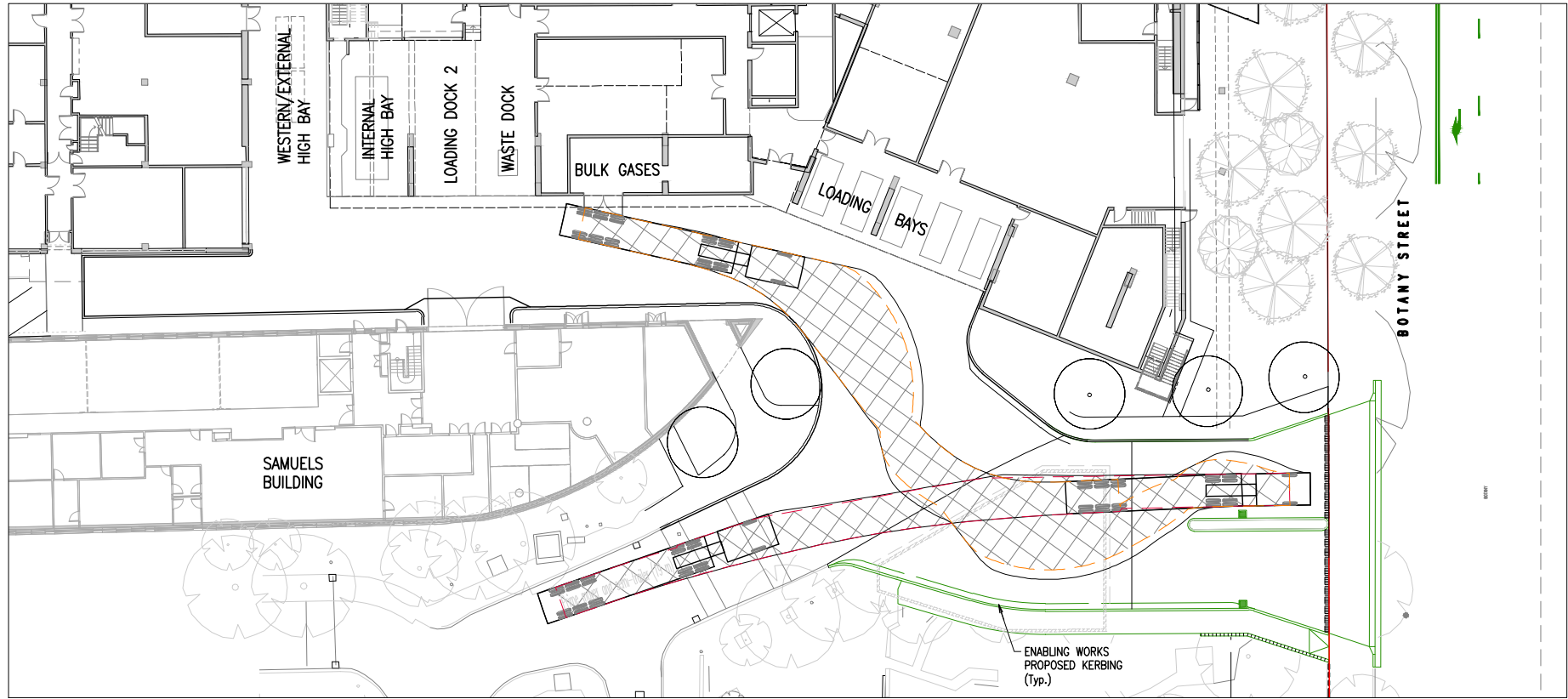
GAS STORAGE – 19m ARTICULATED VEHICLE – ACCESS MANOEUVRE
