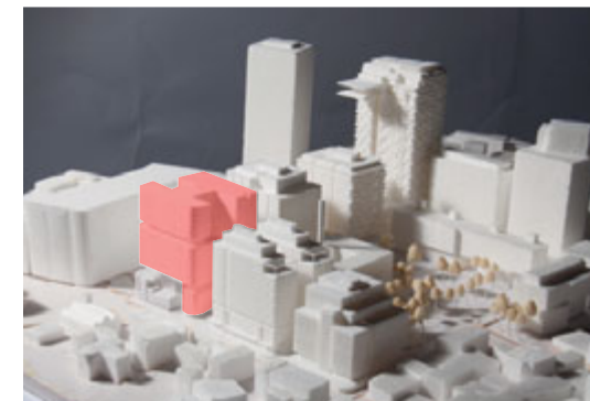
03. Block 4N: Version 3 One Block with stepped back centre part to create strong vertical emphasis on Broadway with flat facade on Abercrombie Street.
