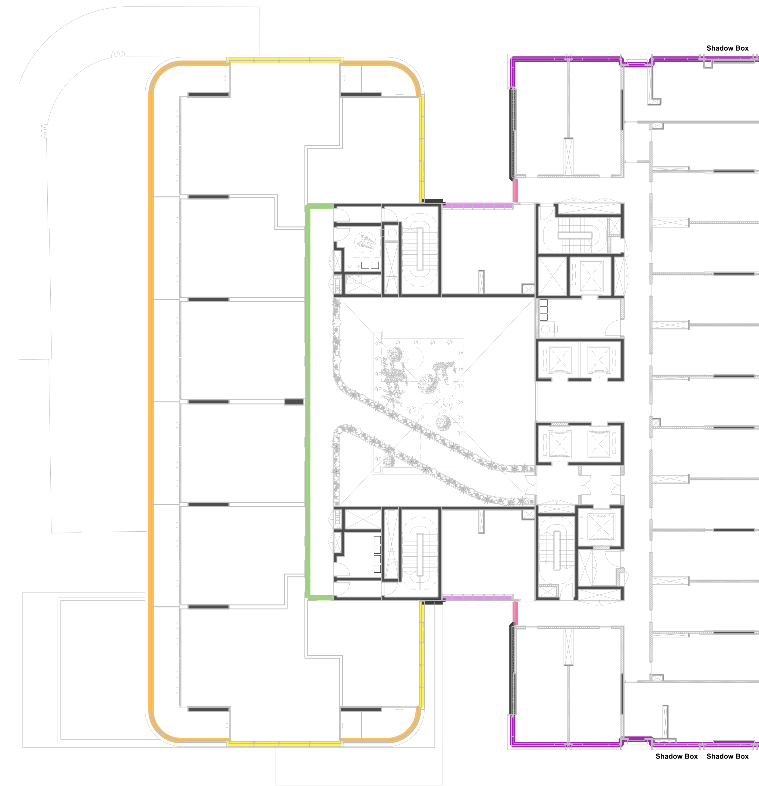
04 Cladding Typologies - Plan Resi (L12-16) / Hotel (L14-18) 1:20
