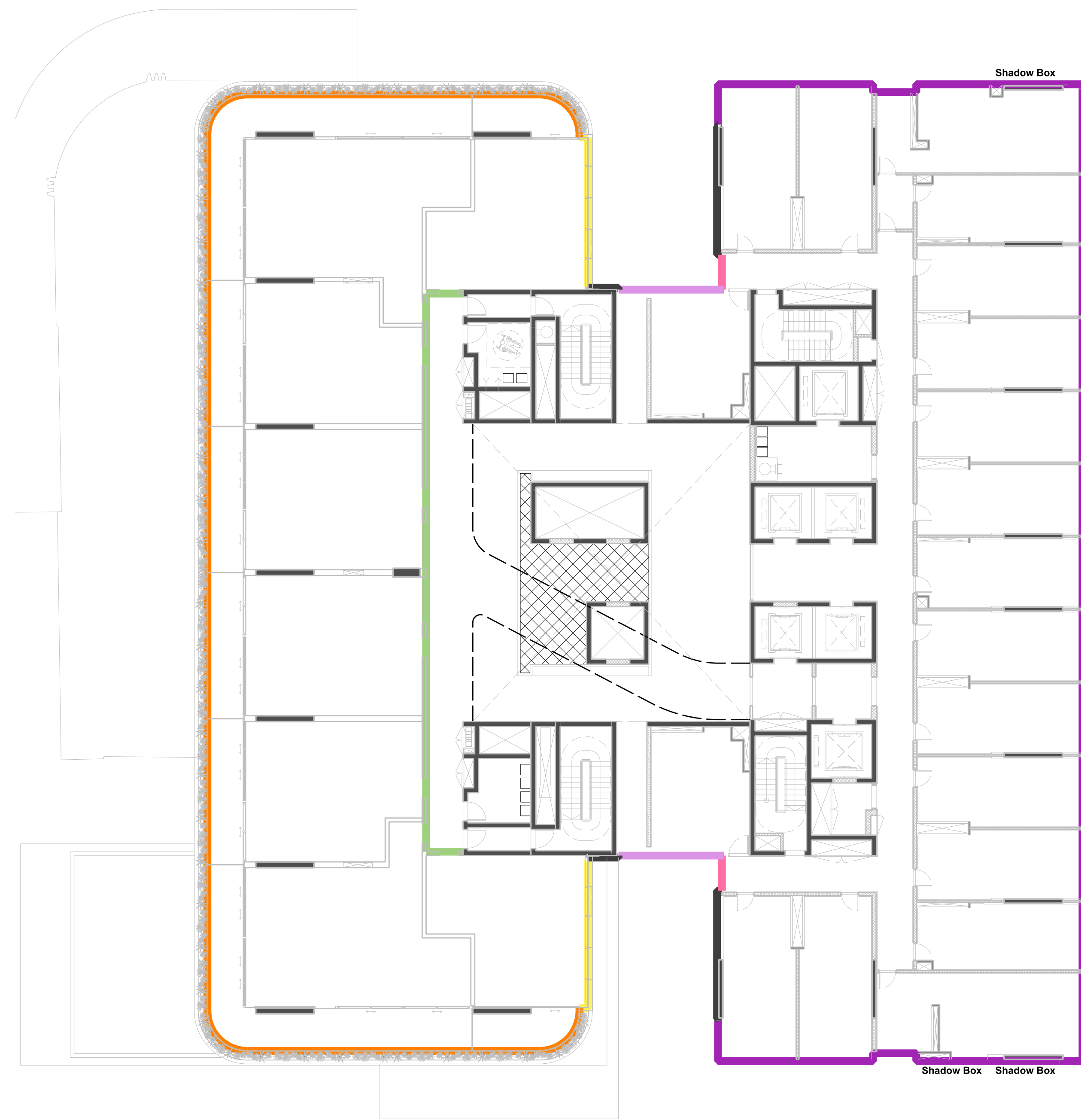
03 Cladding Typologies - Plan Resi (L11) / Hotel (L13) 1:20
