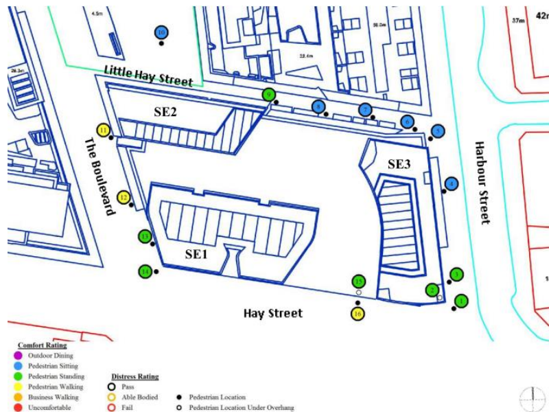
Figure 7: Pedestrian wind speed measurement locations with comfort/distress ratings Boulevard
