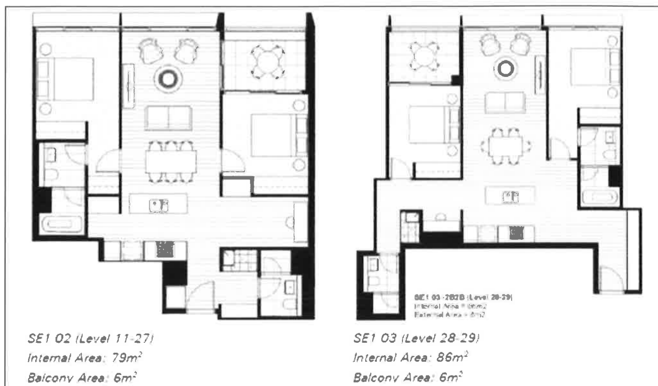
Figure 14: Example of two bedroom apartments with non-compliant balconies (Source: Applicant's RfS)
