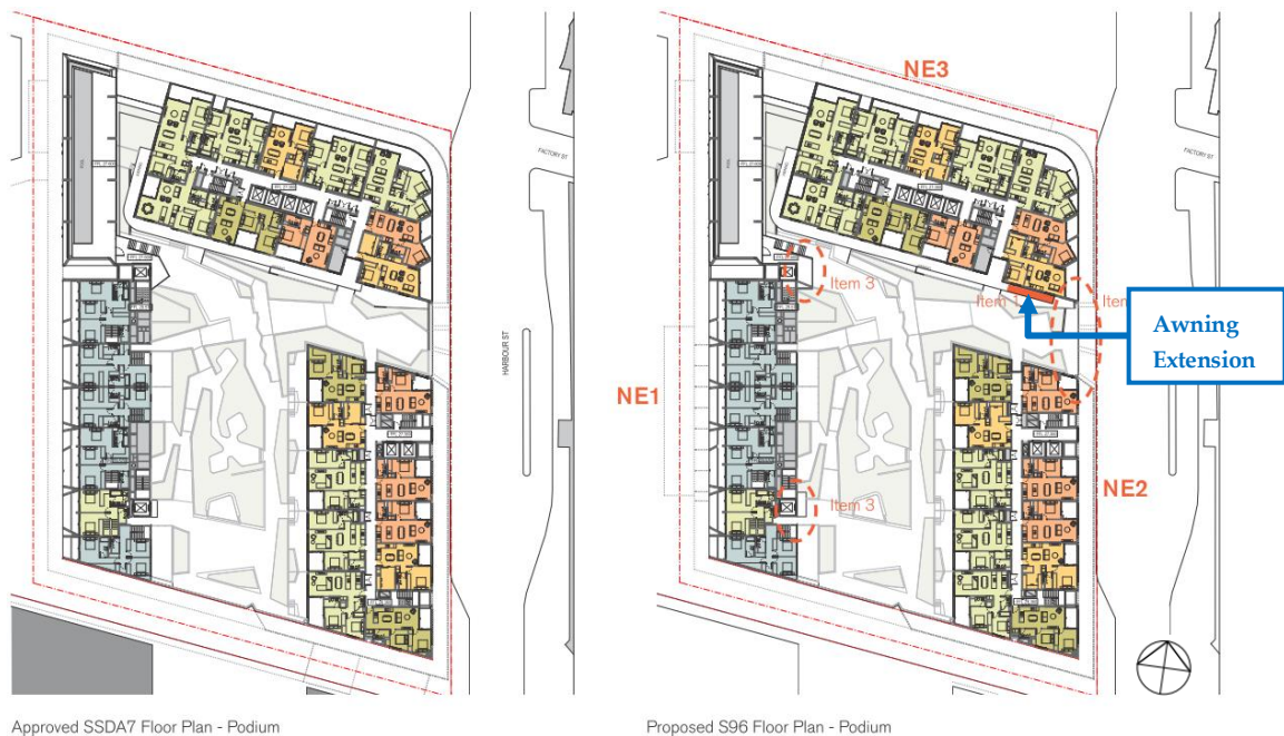
Figure 1: Approved SSDA7 Podium Floor Plan (L), Proposed S96 Podium Floor Plan (R)
